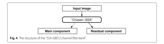
To demonstrate, the "Octagon" input image was processed with the "SSA-iSBD 2-channel filter bank," where 2D-SSA is used as "chosen-SSA," which can be also called "2D-SSA-iSBD 2-channel filter bank," with the window sizes  $(L_x, L_y) = (10, 10)$  and (30, 30). The resulting main and residual component are shown in Fig. 5.
