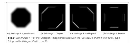
Noticeably, the *sub-images 2* and *sub-images 3* created with both exemplary filter banks highlight not only the desired directional components, but they also provide slightly visible traces of the directional components contained in *sub-images 4*.
