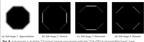
**Fig. 8** Sub-images 1–4 of the "Octagon" image processed with the "SSA-iSBD 4-channel filter bank," type "vertical/horizontal" with L=30
