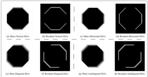
**Fig. 6** These main and residual components show the "Octagon" image processed with "SSA-iSBD 2-channel filter bank" with following types of "chosen-SSA": "Vertical-SSA," "Horizontal-SSA," "Diagonal-SSA," and "Antidiagonal-SSA"
