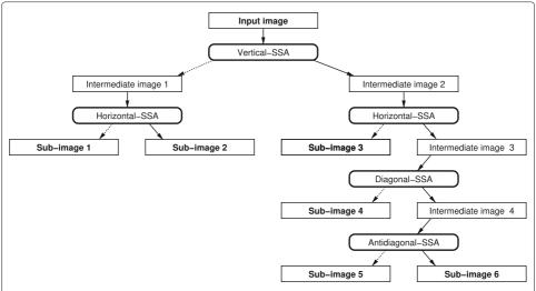
**Fig. 10** The structure of the "SSA-iSBD 6-channel filter bank" implemented as an extension of the "SSA-iSBD 4-channel filter bank," type "vertical/horizontal"
