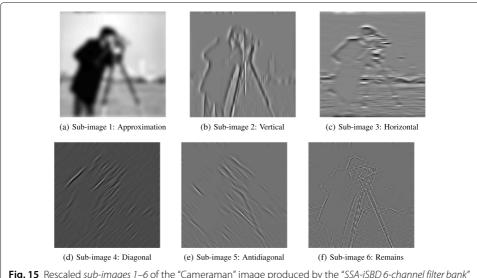
**Fig. 15** Rescaled *sub-images 1–6* of the "Cameraman" image produced by the "SSA-iSBD 6-channel filter bank" with L=12
