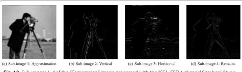
**Fig. 12** Sub-images 1-4 of the "Cameraman" image processed with the "SSA-iSBD 4-channel filter bank," type "vertical/horizontal," with L=4
