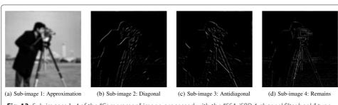
**Fig. 13** Sub-images 1–4 of the "Cameraman" image processed with the "SSA-iSBD 4-channel filter bank," type "diagonal/antidiagonal," with L=4
