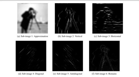
**Fig. 14** The sub-images 1–6 of the "Cameraman" image produced by the "SSA-iSBD 6-channel filter bank" with L=12
