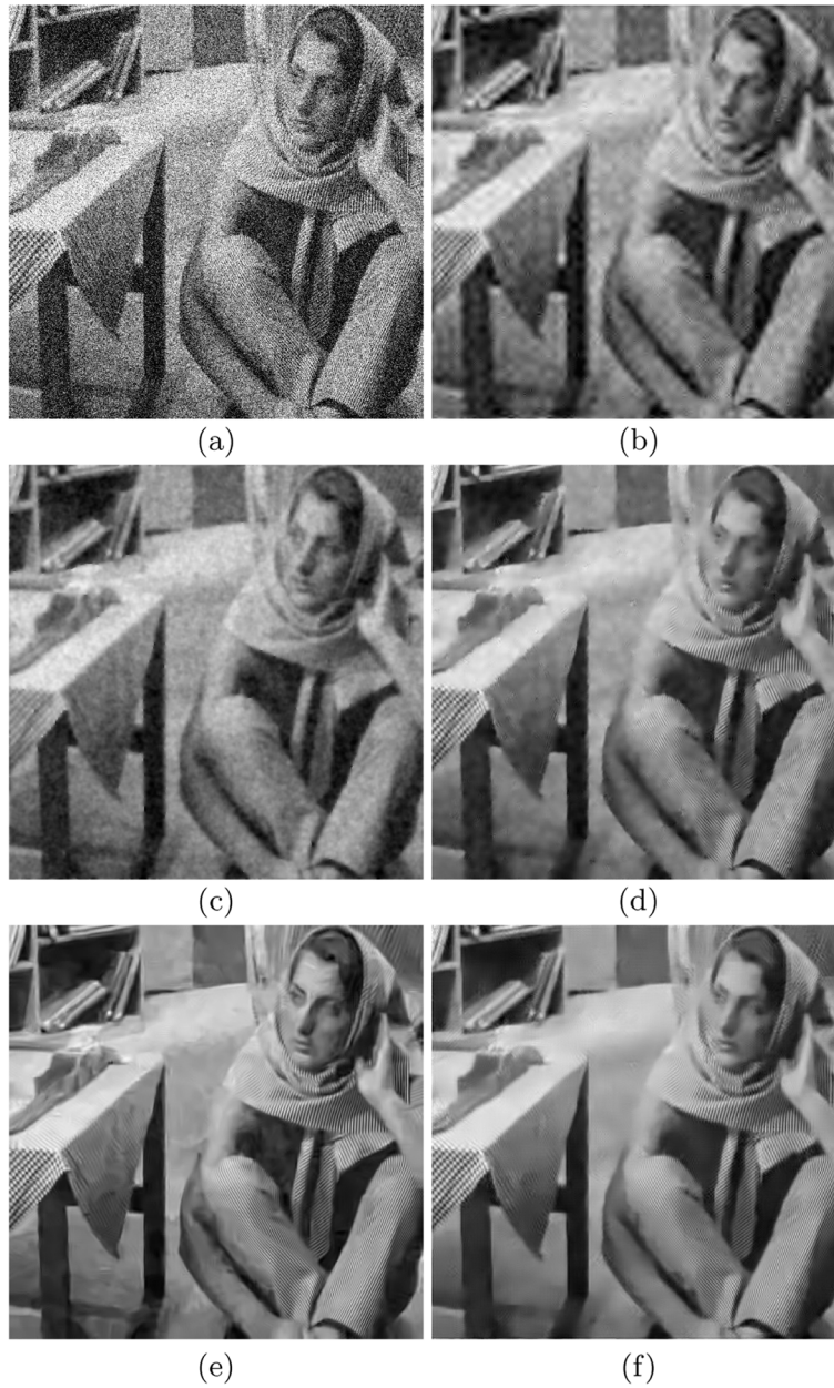
Fig. 7 Denoising performance comparisons of “Barbara” with the noise deviation \sigma = 50 by different methods. a Noisy image. b Denoised image by wavelet thresholding. c Denoised image by TV. d Denoised image by K-SVD. e Denoised image by BM3D. f Denoised image by the proposed method
