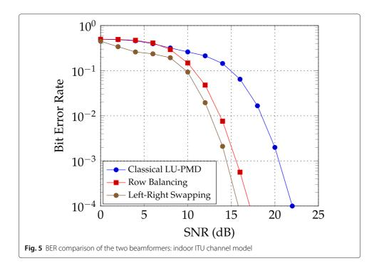
Significant improvement is obtained with the proposed method in both MIMO  $3\times3$  contexts: indoor (5) and outdoor (6). Observe how the performance gain is very important in the more severe outdoor context. For example, the same BER level of  $10^{-3}$  is reached with the proposed solution with about 5 dB drop in SNR compared to the "row balancing" trick. This is due to the fact that the post-filter matrix is better conditioned now, while the output filtering power remains reasonably high.
