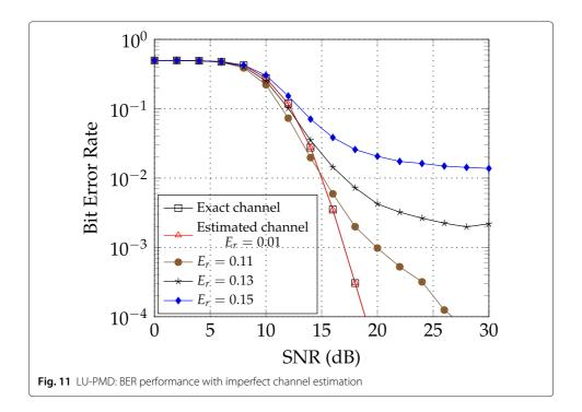
In the sequel, we compute the pre- and post-filters from the decomposition of  $\widehat{H}(z)$  but the MIMO transmission system is still simulated using the exact channel matrix H(z). QR-based decomposition is also implemented in this channel-pre/post-filter mismatch setting for comparison. We evaluate the BER performance for different values of the relative error  $E_r = E/\|H(z)\|_2$ . The results are presented in Figs. 11 and 12.
