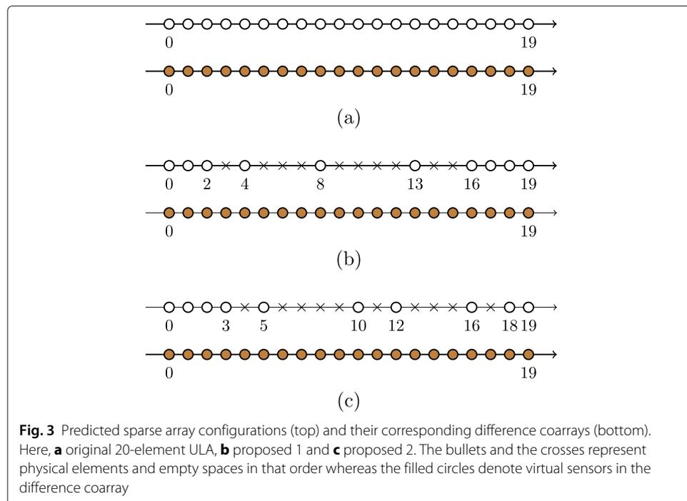
**Fig. 3** Predicted sparse array configurations (top) and their corresponding difference coarrays (bottom). Here, **a** original 20-element ULA, **b** proposed 1 and **c** proposed 2. The bullets and the crosses represent physical elements and empty spaces in that order whereas the filled circles denote virtual sensors in the difference coarray
