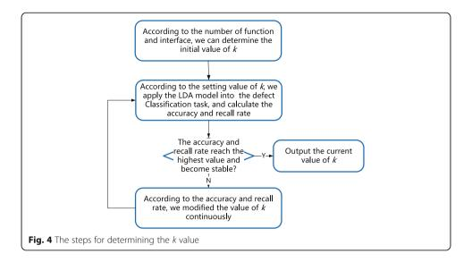
based on the accuracy and recall rate until the classification accuracy and recall rate reach the highest value and become stable, at which time the current k value is considered to be the optimal value for the radar project in the current field.
