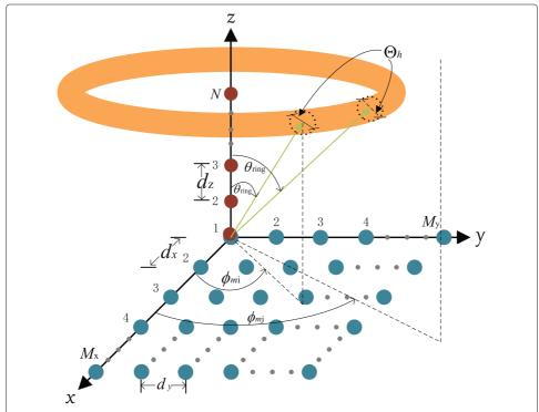
**Fig. 1** The linear array is arranged on the *z*-axis, and its donut-shaped steered main beam is approximated by several steering beams of a virtual planar array on the *x*-*y* plane
