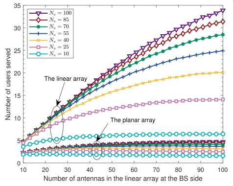
**Fig. 5** Comparison of the number of simultaneous users served by benchmark Algorithm 1 when the BS side is equipped with a linear array and a planar array, respectively
