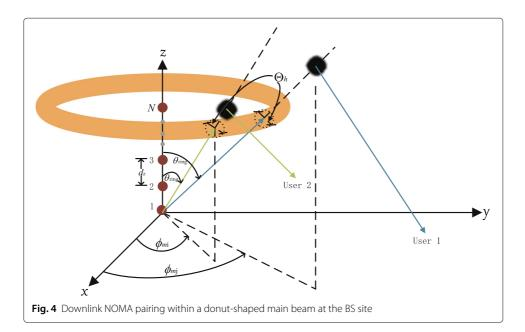
beam has two scatterers in its donut-shaped main beam direction, and the corresponding two channel clusters are scattered and directed toward the far user 1 and the near user 2, respectively. The average received energy in the corresponding scattering cluster is smaller for user 1 due to the longer path experienced by the scattering path and the fact that the energy of the longer path is more absorbed in the atmosphere.
