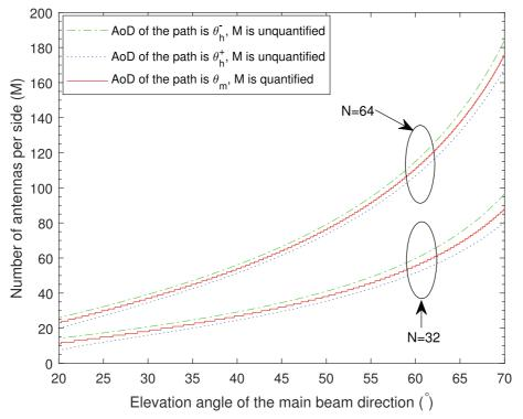
**Fig. 2** The main direction of the steering beam of a linear array versus the number of elements per side of a virtual planar antenna array
