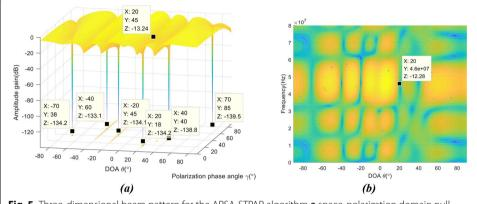
Fig. 5 Three-dimensional beam pattern for the APSA-STPAP algorithm a space-polarization domain null pattern and **b** top view of the space-time domain null pattern
