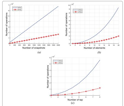
**Fig. 9** Computational complexity of the APSA-STPAP and DPSA-STPAP algorithms **a** number of operations versus the number of samples, **b** number of operations versus the number of array elements, and **c** number of operations versus the number of time domain taps
