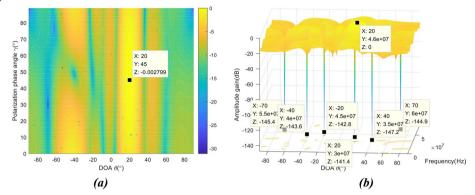
**Fig. 7** Three-dimensional beam pattern for the APSA-STPAP algorithm **a** space-polarization domain null pattern and **b** top view of the space-time domain null pattern
