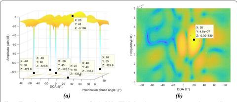
Fig. 6 Three-dimensional beam pattern for the DPSA-STPAP algorithm a space-polarization domain null pattern and **b** top view of the space-time domain null pattern
