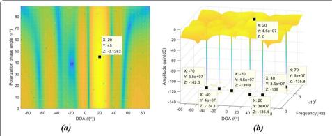
**Fig. 8** Three-dimensional beam pattern for the DPSA-STPAP algorithm **a** space-polarization domain null pattern and **b** top view of the space-time domain null pattern
