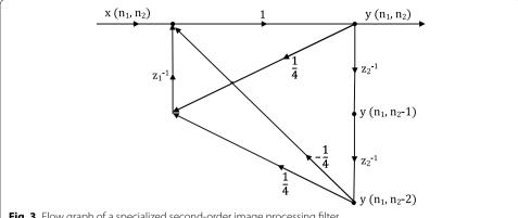
Fig. 3 Flow graph of a specialized second-order image processing filter
