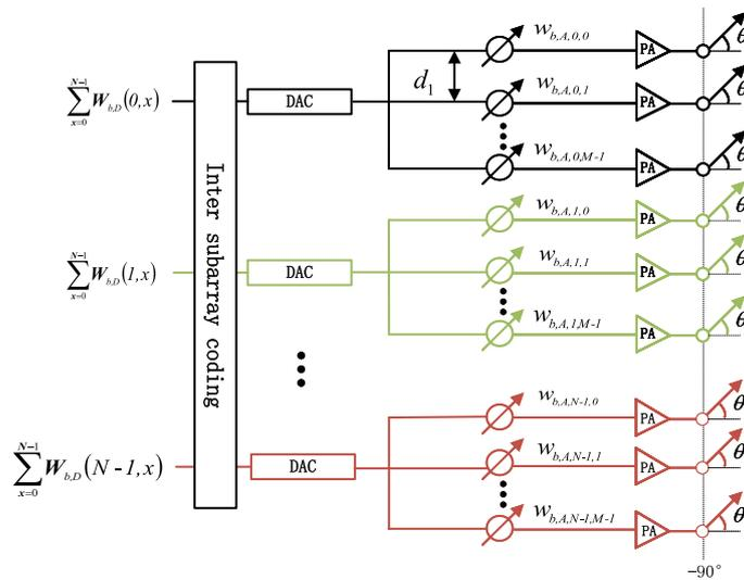
**Fig. 2** Hybrid beamforming structure based on localized subarrays
