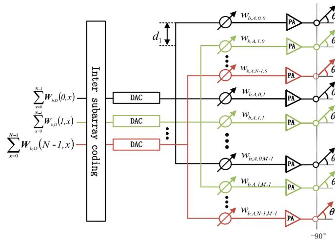
**Fig. 1** Hybrid beamforming structure based on interleaved subarrays
