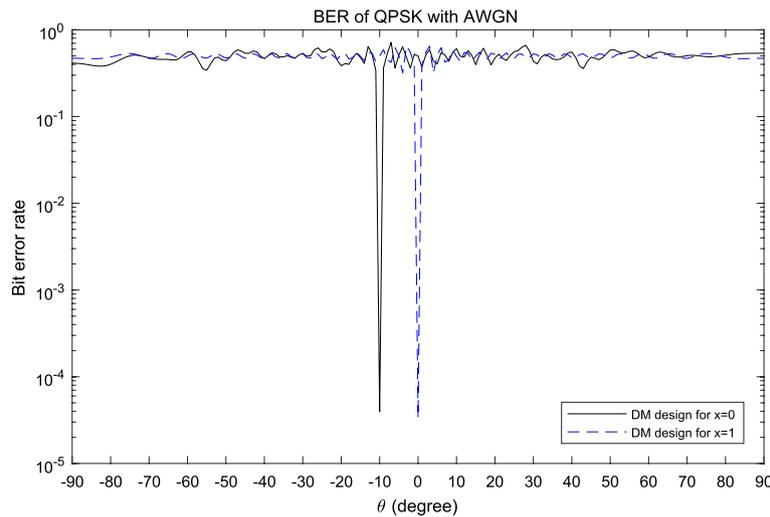
Fig. 6 Spatial distribution of BER for dual-beam multiplexing
