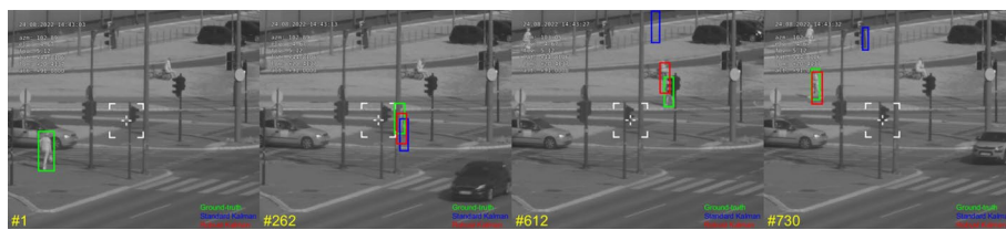
Fig. 9 The first test video sequence. Pedestrian tracking in scenario with partial and full static occlusions. Comparison of bounding boxes obtained by standard Kalman filter (blue box) and robust Kalman filter (red box) to ground-truth (green box) bounding box
