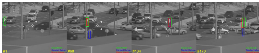
Fig. 10 The second test video sequence. Pedestrian tracking in scenario with partial moving and full static occlusions. Comparison of bounding boxes obtained by standard Kalman filter (blue box) and robust Kalman filter (red box) to ground-truth (green box) bounding box
