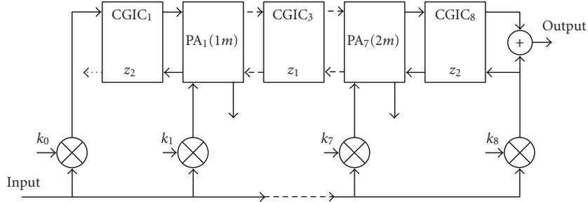
FIGURE 2: Second-order CGIC-PA rotated digital filter structure.
