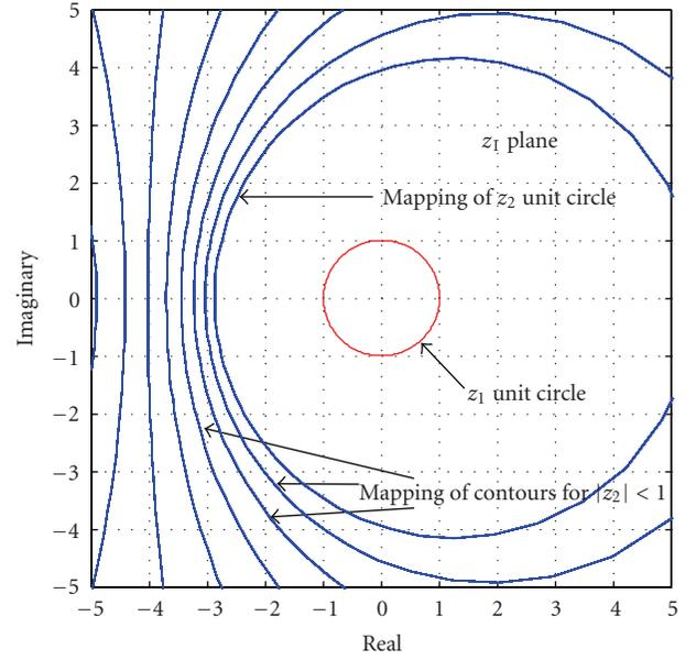
FIGURE 4: Mapping of  $z_2$  unit circle onto  $z_1$  plane for the stable filter.
