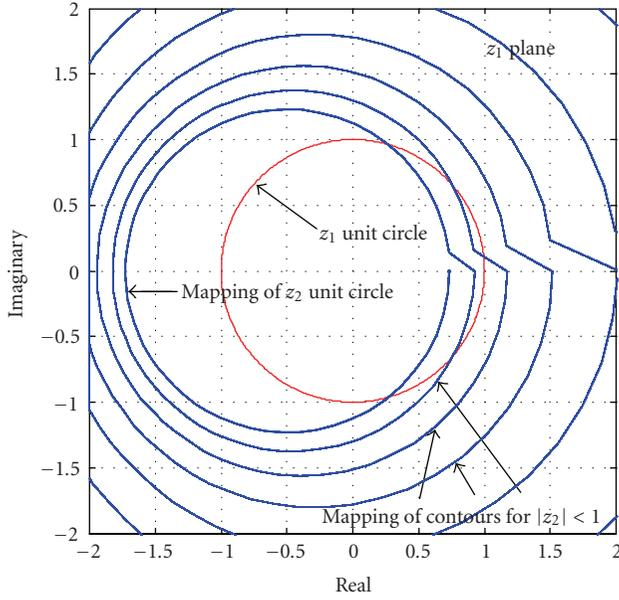
FIGURE 3: Mapping of  $z_2$  unit circle onto  $z_1$  plane for the unstable filter.
