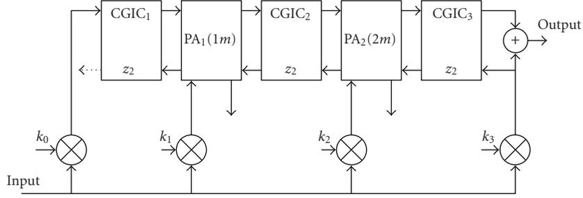
FIGURE 1: First-order CGIC-PA rotated digital filter structure.
