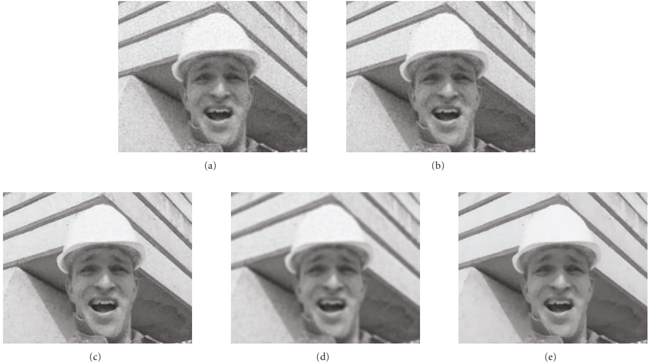
FIGURE 13: Experimental results in the nonsynthetic “noise” case. (a) LR frame, (b) Laplacian SR result with \lambda = 0.128 , (c) TV SR result with \lambda = 2.048 , (d) Laplacian SR result with \lambda = 2.048 , and (e) TV SR result with \lambda = 4.096 .
