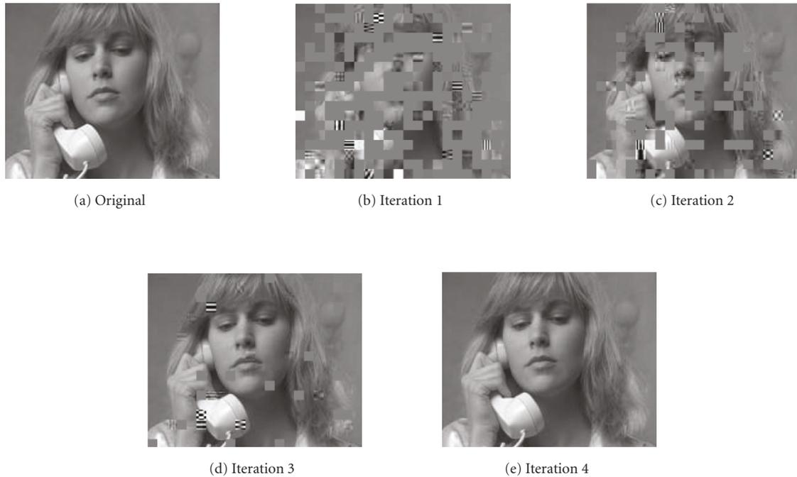
FIGURE 11: Original and decoded “Suzie” images over AWGN channel using proposed asymmetric turbo code with interleaver with an  $E_b/N_0$  of 2 dB.
