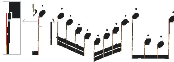
FIGURE 8: Vertical segment detection . In light blue the black pixels added through vertical closing, in orange the main black run and in red the run extensions corresponding to the merged black runs.
