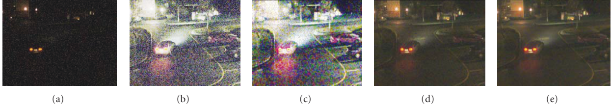
FIGURE 9: Underexposed video results. (a) Test video added by impulse ( p = 10\% ) noise. (b) Result of histogram equalization. (c) Result of ASTA filter followed by histogram equalization. (d) Result of ASTA system. (e) Result of our system.
