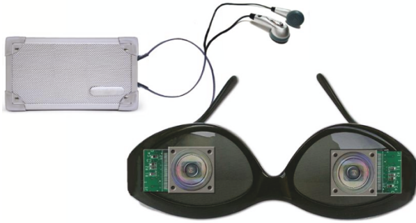
FIGURE 11: Anticipated embedded stereo vision system.
