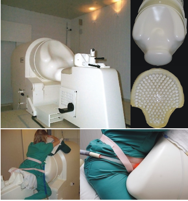
FIGURE 1: Multichannel superconducting quantum interference device (SQUID) system.
