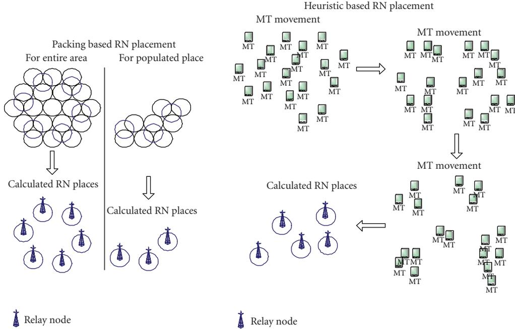
FIGURE 3: Packing-based RN placement and heuristic RN placement.
