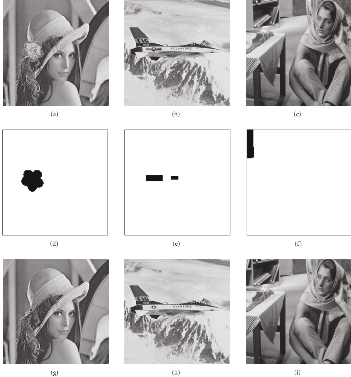
FIGURE 7: The collage attack experiments: (a) a tampered version of Lena^{(W)} ; (b) a tampered version of Jet^{(W)} ; (c) a tampered version of Barbara^{(W)} , respectively; (g)–(i) the images recovered from (a)–(c), respectively. The PSNR values are 41.58 dB for (g); 42.45 dB for (h); and 43.01 dB for (i).
