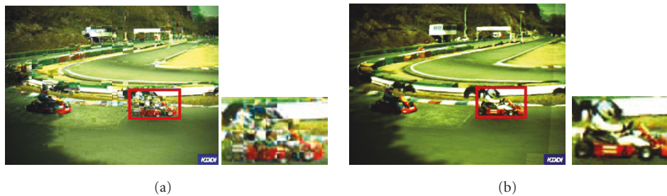
FIGURE 16: Side information generation from (a) the temporal direction, (b) from the view direction with the graph-based matching.
