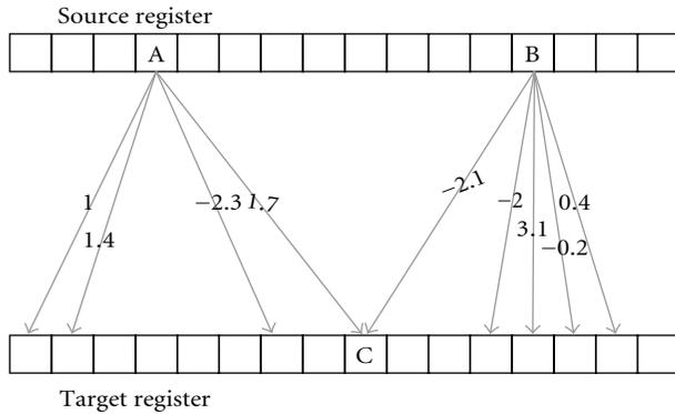
FIGURE 3: Linkmaps allow multiplicative connections between the processing cells. Each cell can be connected to any other cell. Here, different linkmaps are shown for cells A and B, where  $C = 1.7A - 2.1B$ .
