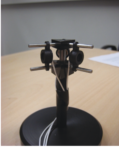
FIGURE 12: Microphone array with 3 outward facing cardioid microphones.
