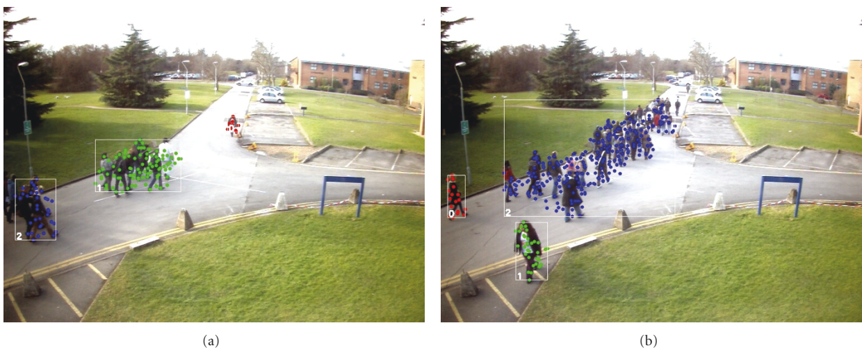
FIGURE 4: Effect of perspective distortion on the number of detected interest points: note how the same woman in (a) is far from the camera (cluster 0, red dots) and only 9 interest points are detected, while in (b) she is closer to the camera (cluster 1, green dots) and 30 interest points are associated to her.
