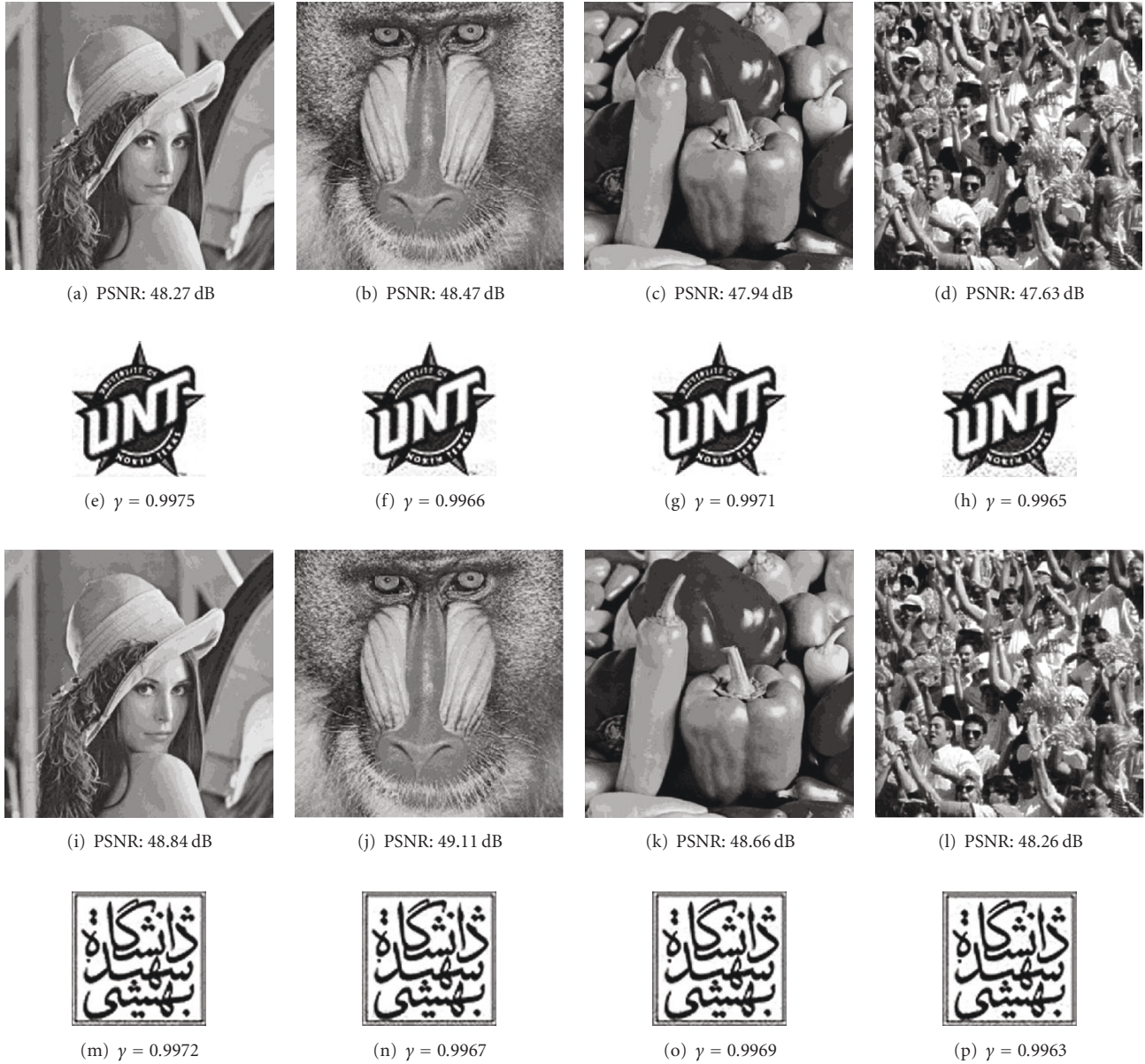
FIGURE 13: (a)–(d) Watermarked images after embedding 256 \times 256 watermark image as shown in Figure 11(b). (e)–(h) Extracted watermarks from (a)–(d), respectively. (i)–(l) Watermarked images after embedding 256 \times 256 watermark image as shown in Figure 11(d). (m)–(p) Extracted watermarks from (i)–(l), respectively.
