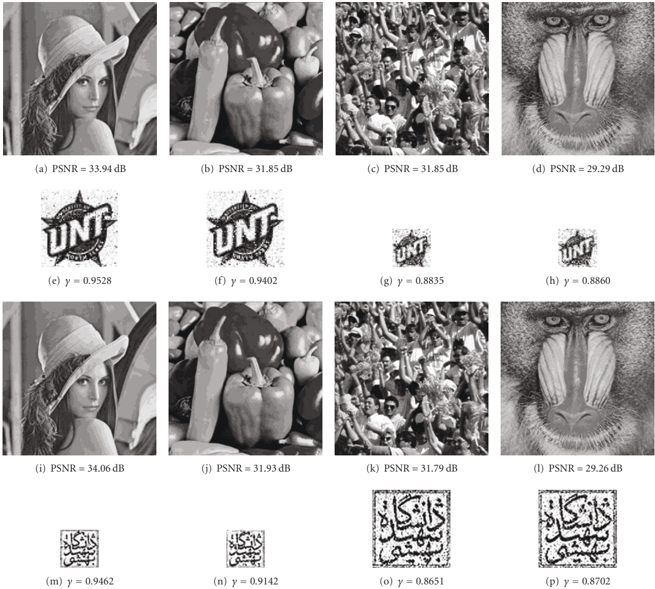
FIGURE 23: (a) and (b) Lena and Peppers watermarked images with 256 \times 256 watermark image as shown in Figure 11(b) after Scaling (1/2), (e) and (f) the extracted watermarks with size 256 \times 256 from (a) and (b), respectively. (c) and (d) Crowd and Baboon watermarked images with 128 \times 128 watermark image as shown in Figure 11(b) after Scaling (1/2), (g) and (h) the extracted watermarks with size 128 \times 128 from (c) and (d), respectively. (i) and (j) Lena and Peppers watermarked images with 128 \times 128 watermark image as shown in Figure 11(d) after Scaling (1/2), (m) and (n) the extracted watermarks with size 128 \times 128 from (i) and (j), respectively. (k) and (l) Crowd and Baboon watermarked images with 256 \times 256 watermark image as shown in Figure 11(d) after Scaling (1/2), (o) and (p) the extracted watermarks with size 256 \times 256 from (k) and (l), respectively.
