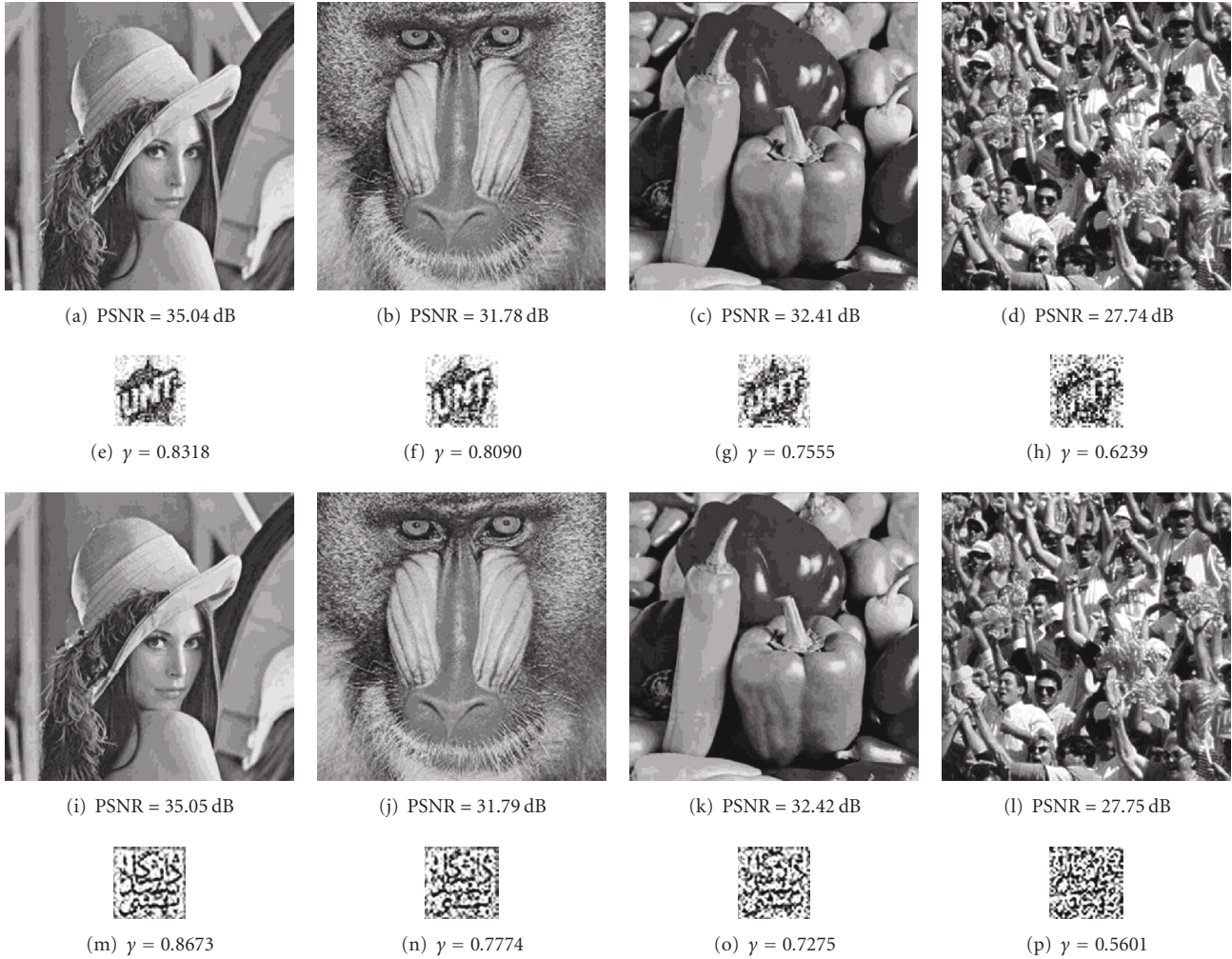
FIGURE 15: (a)–(d) The watermarked Lena, Baboon, Peppers and Crowd images with 128 \times 128 watermark image as shown in Figure 11(b) after JPEG compression with quality factor 40%, 30%, 20% and 10%, respectively. (e)–(h) The extracted watermarks ( 128 \times 128 ) from (a)–(d), respectively. (i)–(l) The watermarked Lena, Baboon, Peppers and Crowd image with 128 \times 128 watermark images as shown in Figure 11(d) after JPEG compression with quality factor 40%, 30%, 20% and 10%, respectively. (m)–(p) The extracted watermarks ( 128 \times 128 ) from (i)–(l), respectively.
