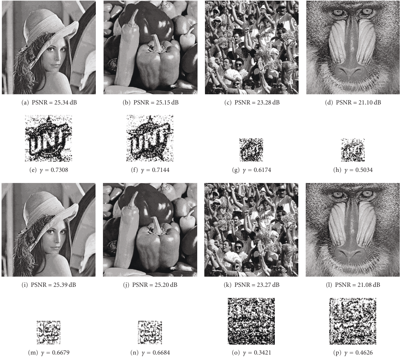
FIGURE 21: (a) and (b) Lena and Peppers watermarked images with 256 \times 256 watermark image as shown in Figure 11(b) after Sharpening, (e) and (f) the extracted watermarks with size 256 \times 256 from (a) and (b), respectively. (c) and (d) Crowd and Baboon watermarked images with 128 \times 128 watermark image as shown in Figure 11(b) after Sharpening, (g) and (h) the extracted watermarks with size 128 \times 128 from (c) and (d), respectively. (i) and (j) Lena and Peppers watermarked images with 128 \times 128 watermark image as shown in Figure 11(d) after Sharpening, (m) and (n) the extracted watermarks with size 128 \times 128 from (i) and (j), respectively. (k) and (l) Crowd and Baboon watermarked images with 256 \times 256 watermark image as shown in Figure 11(d) after Sharpening, (o) and (p) the extracted watermarks with size 256 \times 256 from (k) and (l), respectively.
