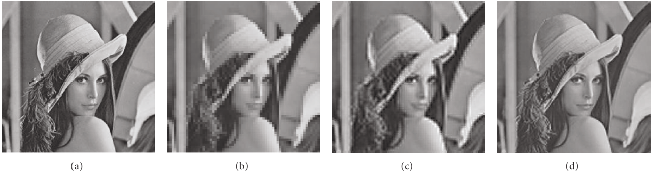
FIGURE 5: (a) Original Lena, (b) Lena created using only DC coefficients of original image, (c) Lena created using estimate formulas (Gonzales method [3]) on image (b), and (d) Lena created using estimate formulas (Veeraswamy method [4]) on image (b).
