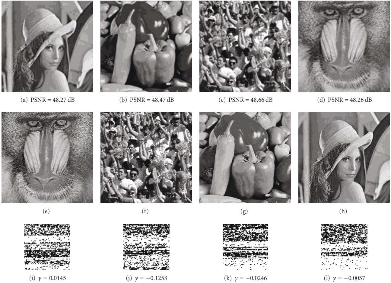
FIGURE 28: (a) and (b) Lena and Peppers watermarked images with 256 \times 256 watermark image as shown in Figure 11(b), (e) and (f) the counterfeit watermarked image with (a) and (b), respectively. (c) and (d) The Crowd and Baboon watermarked images with 256 \times 256 watermark image as shown in Figure 11(d), (g) and (h) the counterfeit watermarked image with (c) and (d), respectively. (i)–(l) the extracted watermark from (e)–(h), respectively.
