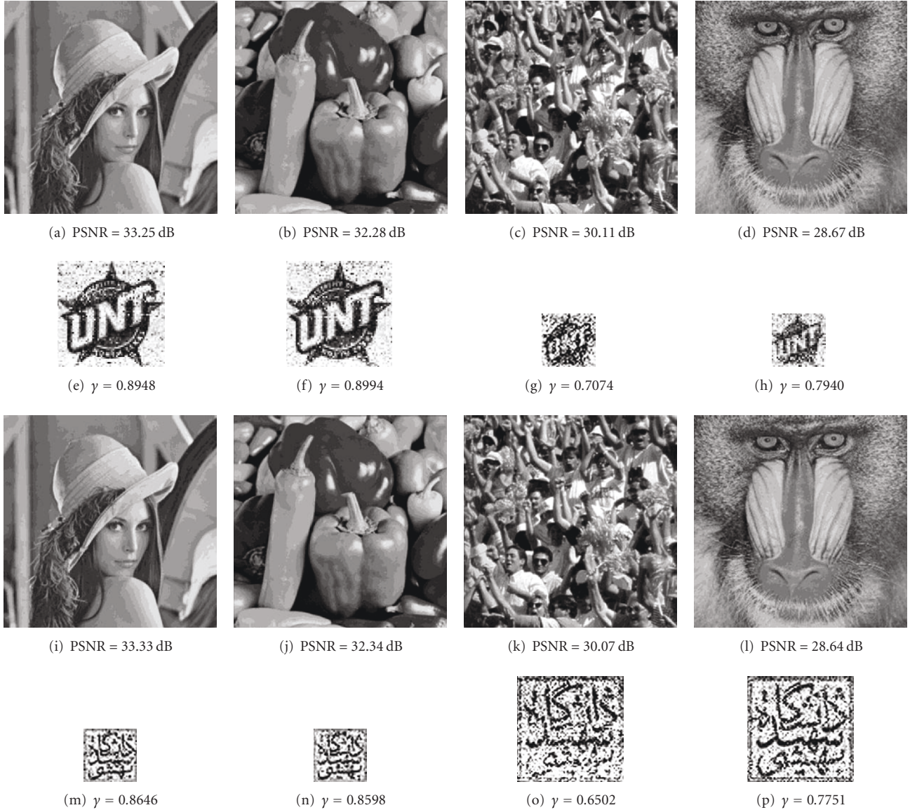
FIGURE 18: (a) and (b) The Lena and Peppers watermarked images with 256 \times 256 watermark image as shown in Figure 11(b) after performing Gaussian lowpass filter with window size 5 \times 5 , (e) and (f) the extracted watermarks with size 256 \times 256 from (a) and (b), respectively. (c) and (d) Crowd and Baboon watermarked images with 128 \times 128 watermark image as shown in Figure 11(b) after performing Gaussian lowpass filter, (g) and (h) the extracted watermarks with size 128 \times 128 from (c) and (d), respectively. (i) and (j) Lena and Peppers watermarked images with 128 \times 128 watermark image as shown in Figure 11(d) after performing Gaussian lowpass filter, (m) and (n) the extracted watermarks with size 128 \times 128 from (i) and (j), respectively. (k) and (l) Crowd and Baboon watermarked images with 256 \times 256 watermark image as shown in Figure 11(d) after performing Gaussian lowpass filter, (o) and (p) the extracted watermarks with size 256 \times 256 from (k) and (l), respectively.
