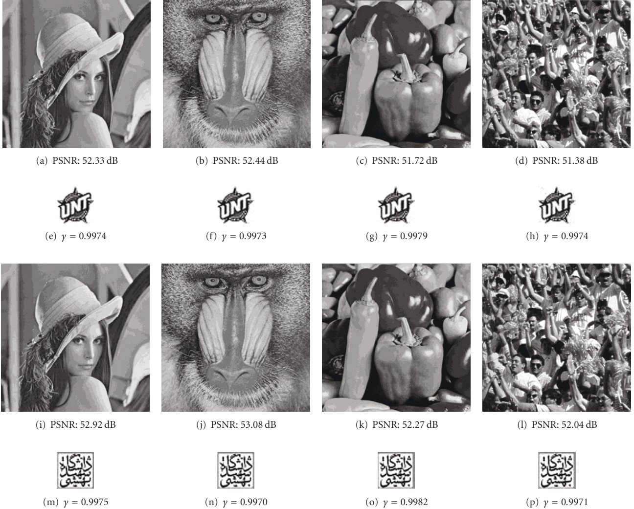
FIGURE 12: (a)–(d) Watermarked images after embedding 128 \times 128 watermark image as shown in Figure 11(b). (e)–(h) Extracted watermarks from (a)–(d), respectively. (i)–(l) Watermarked images after embedding 128 \times 128 watermark image as shown in Figure 11(d). (m)–(p) Extracted watermarks from (i)–(l), respectively.
