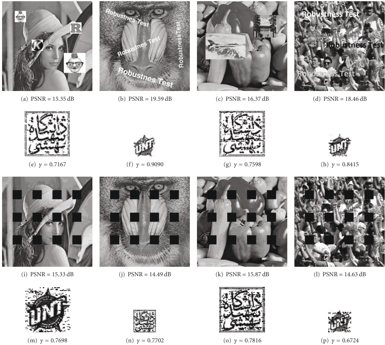
FIGURE 27: (a)–(d) The watermarked Lena, Baboon, Peppers and Crowd images after tampering, respectively. (e)–(h) The extracted watermarks from (a)–(d), respectively. (i)–(l) The watermarked Lena, Baboon, Peppers and Crowd images after data blocks removal, respectively. (m)–(p) The extracted watermarks from (i)–(l), respectively.
