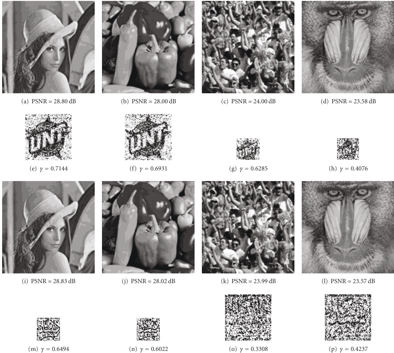
FIGURE 24: (a) and (b) Lena and Peppers watermarked images with 256 \times 256 watermark image as shown in Figure 11(b) after Scaling (1/4), (e) and (f) the extracted watermarks with size 256 \times 256 from (a) and (b), respectively. (c) and (d) Crowd and Baboon watermarked images with 128 \times 128 watermark image as shown in Figure 11(b) after Scaling (1/4), (g) and (h) the extracted watermarks with size 128 \times 128 from (c) and (d), respectively. (i) and (j) Lena and Peppers watermarked images with 128 \times 128 watermark image as shown in Figure 11(d) after Scaling (1/4), (m) and (n) the extracted watermarks with size 128 \times 128 from (i) and (j), respectively. (k) and (l) Crowd and Baboon watermarked images with 256 \times 256 watermark image as shown in Figure 11(d) after Scaling (1/4), (o) and (p) the extracted watermarks with size 256 \times 256 from (k) and (l), respectively.
