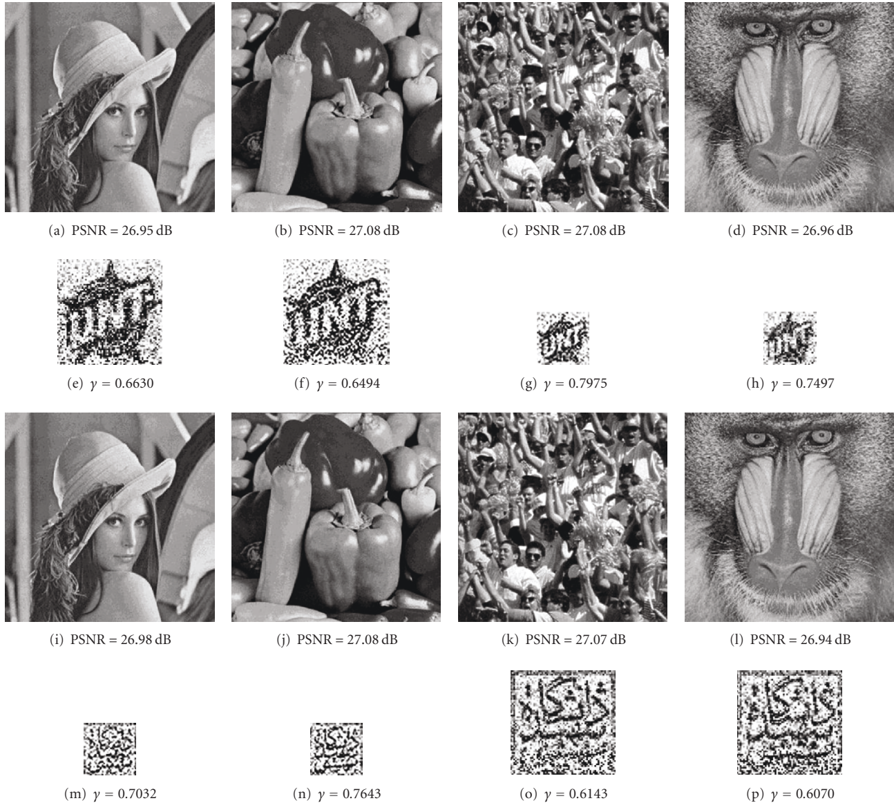
FIGURE 17: (a) and (b) Lena and Peppers watermarked images with 256 \times 256 watermark image as shown in Figure 11(b) after adding Gaussian noise with mean = 0 and variance = 0.002, (e) and (f) the extracted watermarks with size 256 \times 256 from (a) and (b), respectively. (c) and (d) Crowd and Baboon watermarked images with 128 \times 128 watermark image as shown in Figure 11(b) after adding Gaussian noise. (g) and (h) The extracted watermarks with size 128 \times 128 from (c) and (d), respectively. (i) and (j) Lena and Peppers watermarked images with 128 \times 128 watermark image as shown in Figure 11(d) after adding Gaussian noise, (m) and (n) the extracted watermarks with size 128 \times 128 from (i) and (j), respectively. (k) and (l) Crowd and Baboon watermarked images with 256 \times 256 watermark image as shown in Figure 11(d) after adding Gaussian noise. (o) and (p) The extracted watermarks with size 256 \times 256 from (k) and (l), respectively.
