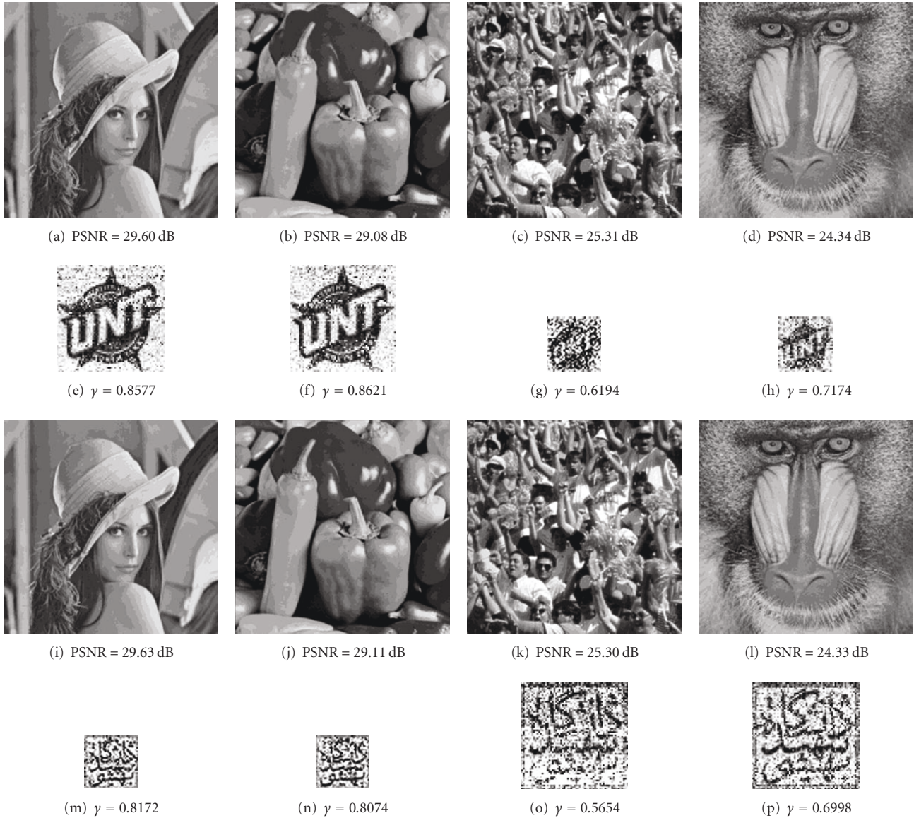
FIGURE 19: (a) and (b) Lena and Peppers watermarked images with 256 \times 256 watermark image as shown in Figure 11(b) after performing Average filter with window size 5 \times 5 , (e) and (f) the extracted watermarks with size 256 \times 256 from (a) and (b), respectively. (c) and (d) Crowd and Baboon watermarked images with 128 \times 128 watermark image as shown in Figure 11(b) after performing Average filter, (g) and (h) the extracted watermarks with size 128 \times 128 from (c) and (d), respectively. (i) and (j) Lena and Peppers watermarked images with 128 \times 128 watermark image as shown in Figure 11(d) after performing Average filter, (m) and (n) the extracted watermarks with size 128 \times 128 from (i) and (j), respectively. (k) and (l) Crowd and Baboon watermarked images with 256 \times 256 watermark image as shown in Figure 11(d) after performing Average filter, (o) and (p) the extracted watermarks with size 256 \times 256 from (k) and (l), respectively.
