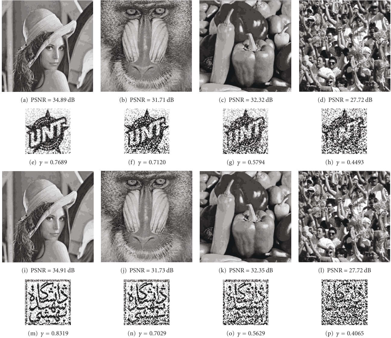
FIGURE 14: (a)–(d) The watermarked Lena, Baboon, Peppers and Crowd images with 256 \times 256 watermark image as shown in Figure 11(b) after JPEG compression with quality factor 40%, 30%, 20% and 10%, respectively. (e)–(h) The extracted watermarks ( 256 \times 256 ) from (a)–(d), respectively. (i)–(l) The watermarked Lena, Baboon, Peppers and Crowd images with 256 \times 256 watermark image as shown in Figure 11(d) after JPEG compression with quality factor 40%, 30%, 20% and 10%, respectively. (m)–(p) The extracted watermarks ( 256 \times 256 ) from (i)–(l), respectively.
