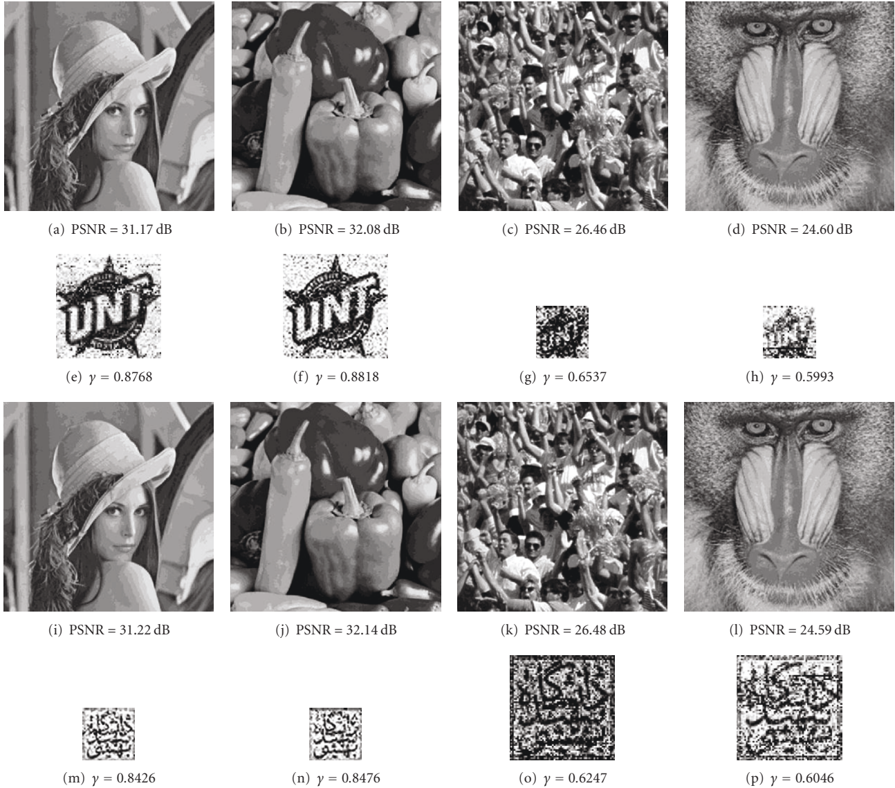
FIGURE 22: (a) and (b) Lena and Peppers watermarked images with 256 \times 256 watermark image as shown in Figure 11(b) after applying Median filter with window size 5 \times 5 , (e) and (f) the extracted watermarks with size 256 \times 256 from (a) and (b), respectively. (c) and (d) Crowd and Baboon watermarked images with 128 \times 128 watermark image as shown in Figure 11(b) after applying Median filter, (g) and (h) the extracted watermarks with size 128 \times 128 from (c) and (d), respectively. (i) and (j) Lena and Peppers watermarked images with 128 \times 128 watermark image as shown in Figure 11(d) after applying Median filter, (m) and (n) the extracted watermarks with size 128 \times 128 from (i) and (j), respectively. (k) and (l) Crowd and Baboon watermarked images with 256 \times 256 watermark image as shown in Figure 11(d) after applying Median filter, (o) and (p) the extracted watermarks with size 256 \times 256 from (k) and (l), respectively.
