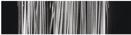
FIGURE 2: CT scan of a sample component. The tight packing of fibers in the material can be clearly seen.
