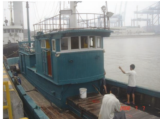
FIGURE 7: The wood-dominant ship for geomagnetic surveying.
