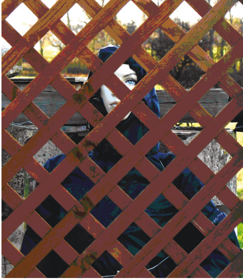
FIGURE 6: Close-up photograph of the upper half of the mannequin positioned at 1 m behind a wooden fence. The scene was scanned at a standoff distance of 325 m in daylight.
