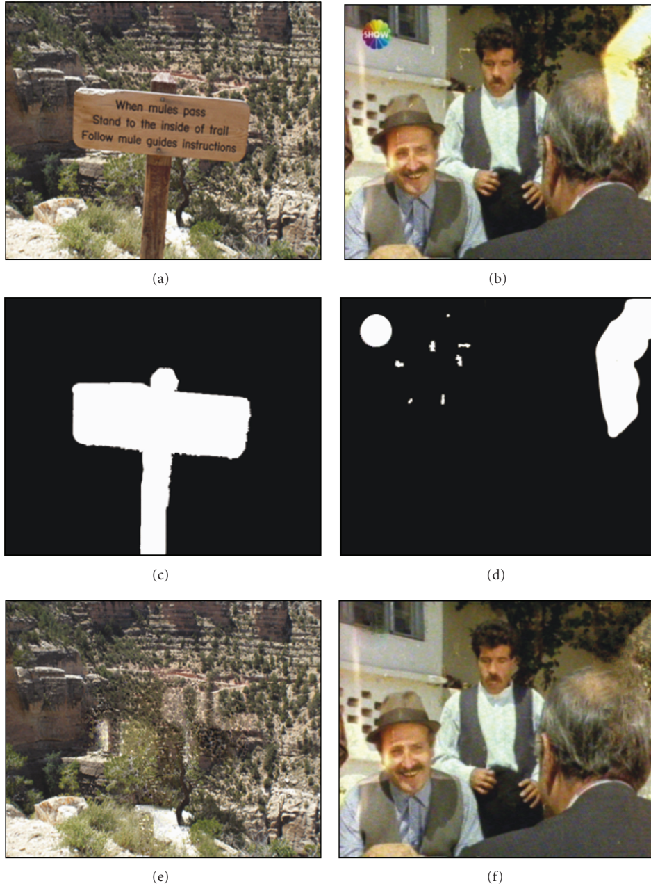
FIGURE 17: The input images (a) and (b) for image completion, the mask images (c) and (d) and output images (e) and (f) are generated by the proposed method.
