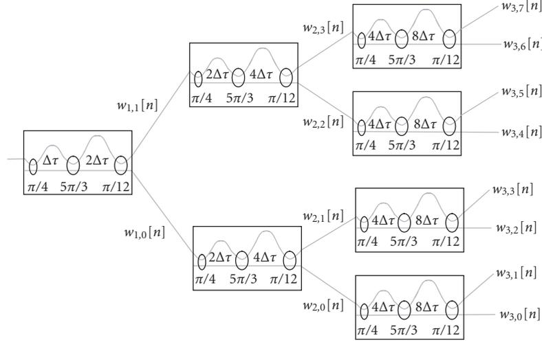
FIGURE 4: Optical architecture for the WP decomposition with Daubechies wavelet filter of length  $M = 4$ . Each optical wavelet filter is a chain of two MZIs, with FSR that decreases from the root to the leaves in a logarithmic way.
