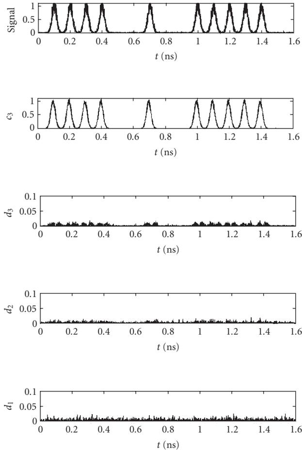
FIGURE 5: Input optical signal at  $B = 10$  Gbps,  $\lambda = 1550$  nm, and SNR = 24 dB; the Gaussian optical pulses have 20 ps width. Scaling coefficients  $c_3$  that coincide with the denoised signal and thresholded detail coefficients at levels 1, 2, 3 are obtained. The DWT is performed with the device of Figure 3, with no subsampling.
