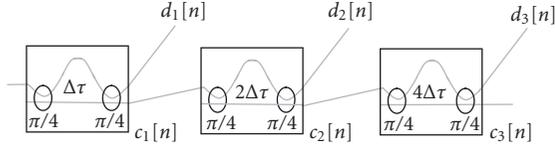
FIGURE 3: Optical architecture for the DWT with Daubechies wavelet of length  $M = 2$ . Each optical wavelet filter is an MZI with input/output 3 dB couplers, and FSR that decreases from the root to the leaves in a logarithmic way.
