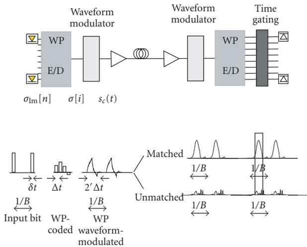
FIGURE 8: Schematic of an optical WPDM system: the data sequences from  $N$  users are WP-encoded by a single optical device; the composite signal is then waveform-modulated by a pulse shaper. The receiver is a reverse version of the transmitter.
