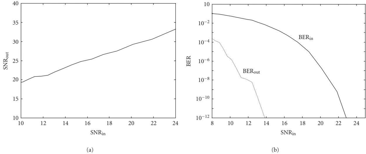
FIGURE 7: (a) SNR of the denoised signal (that coincides with the scaling coefficients  $c_3$  from the device of Figure 3) versus the SNR of the input optical signal. (b) Bit error rate of the input signal (solid line) and the denoised signal (dotted line) versus the SNR of the input signal.
