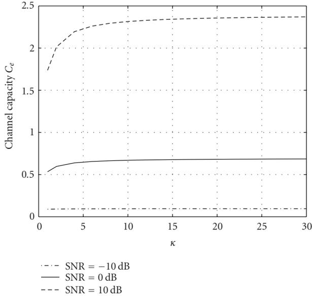
FIGURE 1: Variation of ergodic channel capacity  $C_e$  (in nats/s/Hz) with the number  $\kappa$  for SISO case.
