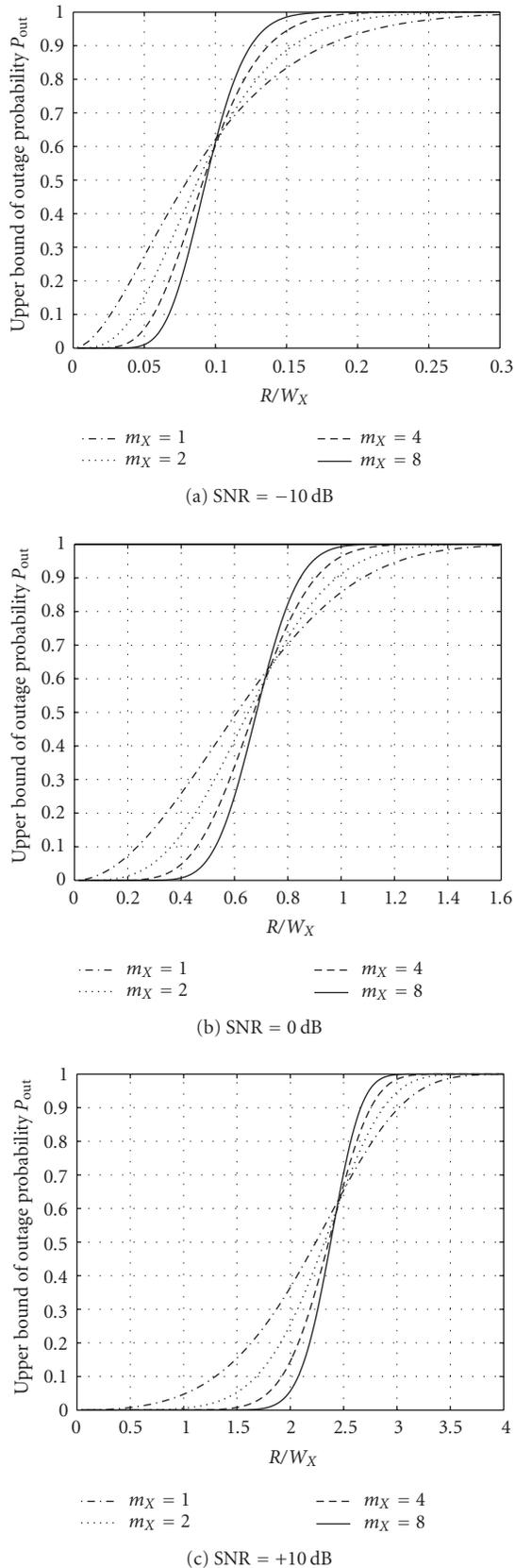
FIGURE 7: The upper bound of the outage probability  $\bar{P}_{\text{out}}$  versus transmission rate  $R/W_X$  (in nats/s/Hz) for various  $m_X$  and SNR for MISO case ( $\kappa = 4$ ).
