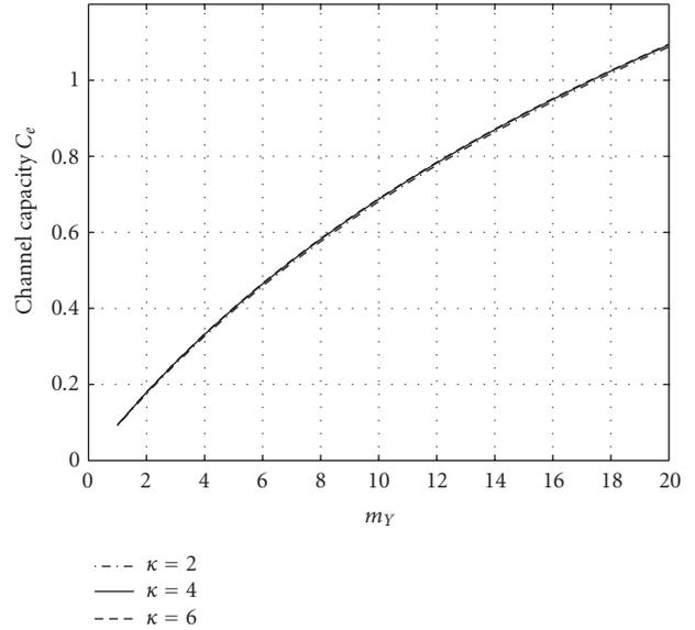
FIGURE 3: Variation of ergodic channel capacity  $C_e$  (in nats/s/Hz) with the number of receive antennas  $m_Y$  for SIMO case (SNR = -10 dB).
