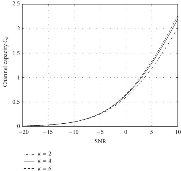
FIGURE 2: Variation of ergodic channel capacity  $C_e$  (in nats/s/Hz) with the ratio SNR (in dB) for SISO case.
