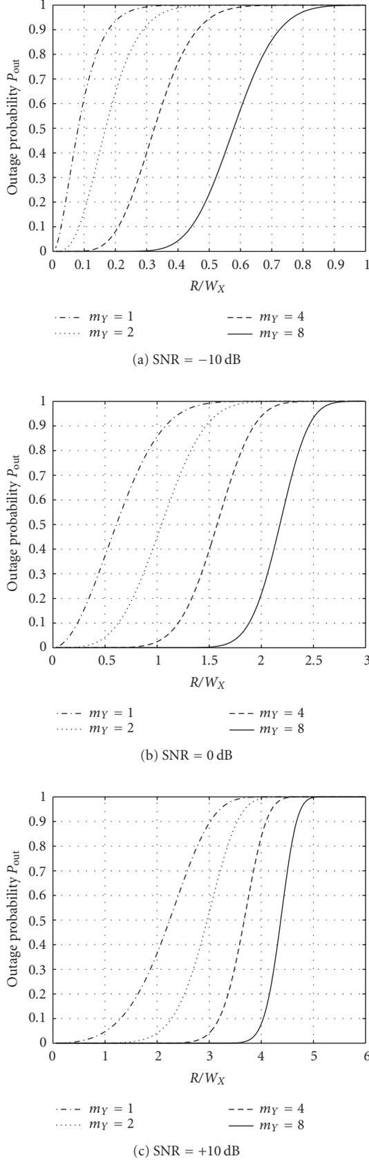
FIGURE 6: Outage probability  $P_{\text{out}}$  versus transmission rate  $R/W_X$  (in nats/s/Hz) for various  $m_Y$  and SNR for SIMO case ( $\kappa = 4$ ).
