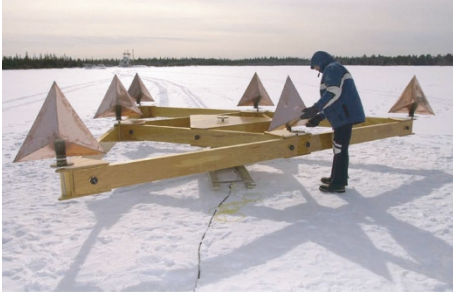
FIGURE 6: The target motion simulator (TMS) experimental apparatus.
