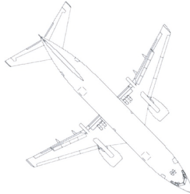
FIGURE 8: Schematic of a Boeing 737 (top view).
