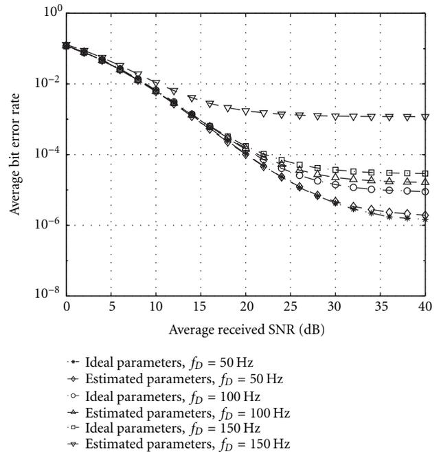
FIGURE 8: Performance comparison of SFBC-OFDM systems with ideal channel parameters and channel parameters estimated by a third order least-square interpolator.
