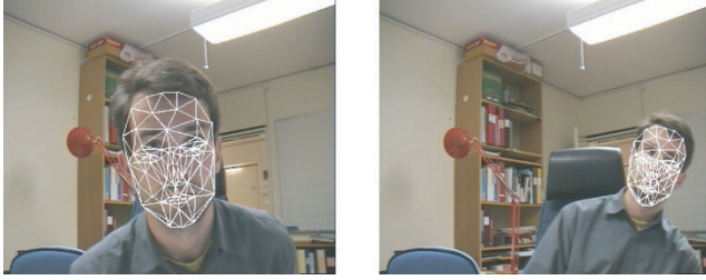
FIGURE 2: Examples of the colour-based algorithm giving a rough initial estimate of the location, size, and inplane rotation of the face.
