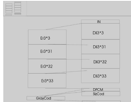
FIGURE 14: The timing diagram generated by SynDEX. The best implementation only uses 2DSPs (root and P1): Er3*3 are treated by the P1 processor and Dil3*3 by the root processor. These functions are executed at the same time. The root processor executes most of other functions. SynDEX indicated (on top) that the efficiency is 1.8 compared to a sequential executive.
