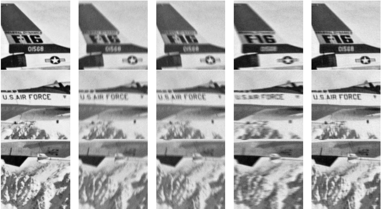
FIGURE 14: F16 image. First column: details of the original image. Second, third, and fourth columns: blurred observations of the original details. Fifth column: restored details (SNR = 20 dB).
