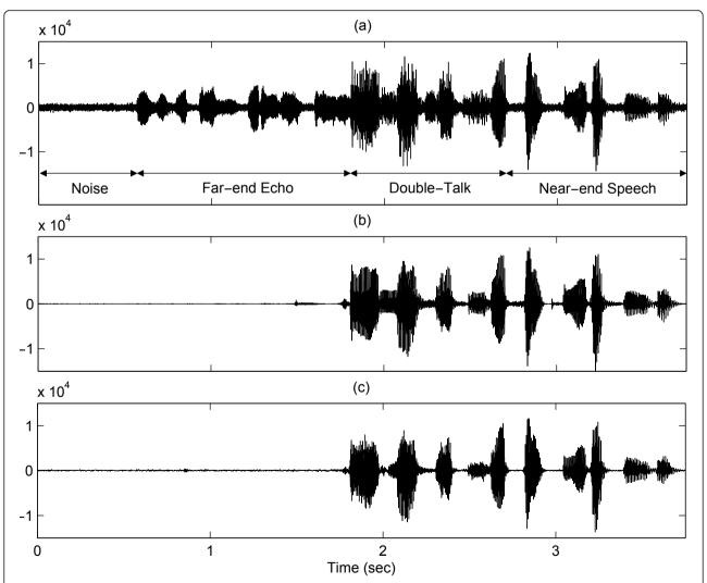
Figure 3 Speech spectrograms (white noise, SNR = 15 dB). (a) Microphone input signal with the noise and echo. (b) Clean near-end speech. (c) Output signal obtained by IS-127+Turbin et al. (d) Output signal obtained by Gustafsson et al. (e) Output signal obtained by the proposed method.
