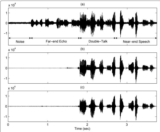
Figure 4 Speech waveforms (white noise, SNR = 15dB). (a) Microphone input signal with the noise and echo. (b) Clean near-end speech. (c) Output signal obtained by the proposed method.
