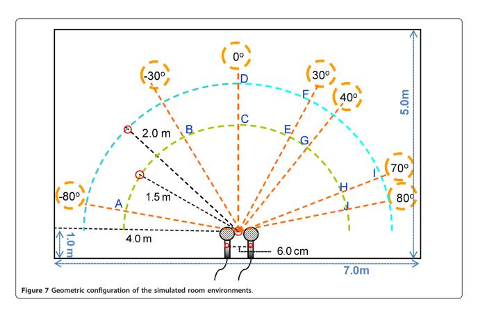
impulse responses were obtained by an image method [1-3] using the above parameters. The impulse responses of the transfer functions from source locations A and H to the two microphones are shown in Figure 8. The peak location was not at the origin because the direct path had its own delay. The filter length was 100
