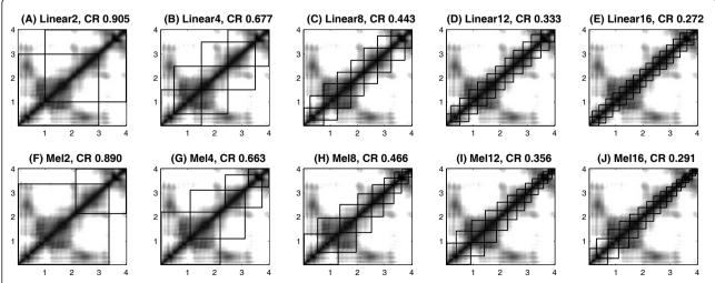
**Figure 9 Various clique designs. (A)-(E)** The center frequencies are linearly scaled, and the clique sizes are equal. **(F)-(J)** The center frequencies and clique sizes are on an inverse mel-scale. The "CR" values are the ratios of the sum of the correlation coefficients included in the cliques to the sum of all of the coefficients.
