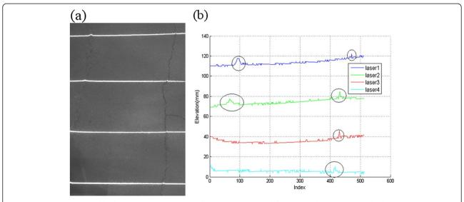
**Figure 2 Pavement scanned by laser stripes.** (a) the stripes from the light source deform across the pavement cracks; (b) the corresponding profile from picture (a), the elevation coordinate for each profile is relative in this Figure.
