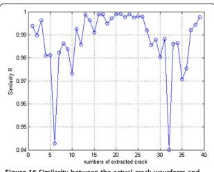
Figure 16 Similarity between the actual crack waveform and the extracted crack waveform.
