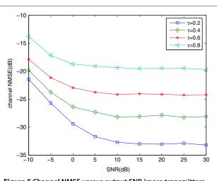
Figure 5 Channel NMSE versus output SNR (more transmitters case).
