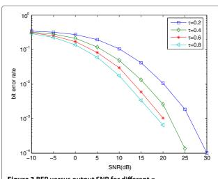
Figure 3 BER versus output SNR for different  $\tau$ .
