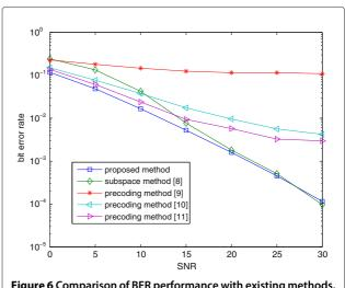
Figure 6 Comparison of BER performance with existing methods.
