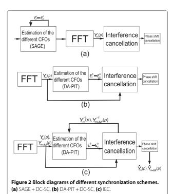
as it allows the iterative cancellation of the ICI and MAI noise [Equations (6) and (7)] during the estimation process. The estimation accuracy is further improved by considering non-consecutive symbols when obtaining the phase shift used by DA-PIT to estimate the CFO.
