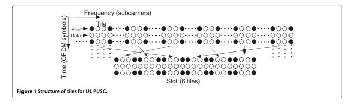
The pilot subcarriers of the three permutation modes are BPSK modulated. In UL O-PUSC and UL AMC, they are transmitted at a boosted power level of 4/3.
