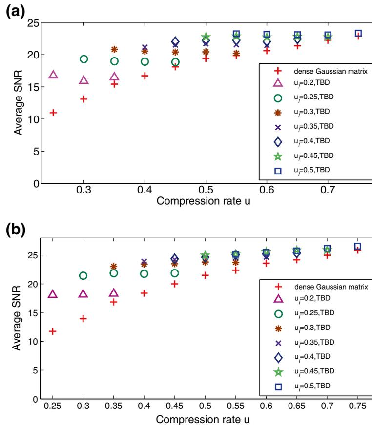
**Figure 13** Average SNR of adaptive quantization of voiced speech signals with different quantization levels: (a)  $Q=32$ . (b)  $Q=64$ .
