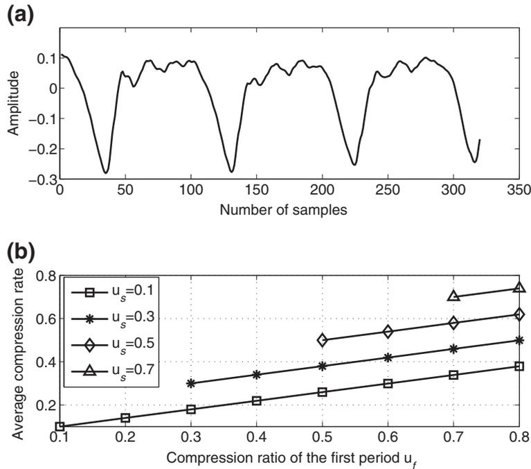
**Figure 3** Waveform of the third type of voiced speech signals and average compression rate: (a) Waveform of the third type of voiced speech signals. (b) Average compression rate with different values of  $u_f$  and  $u_s$ .
