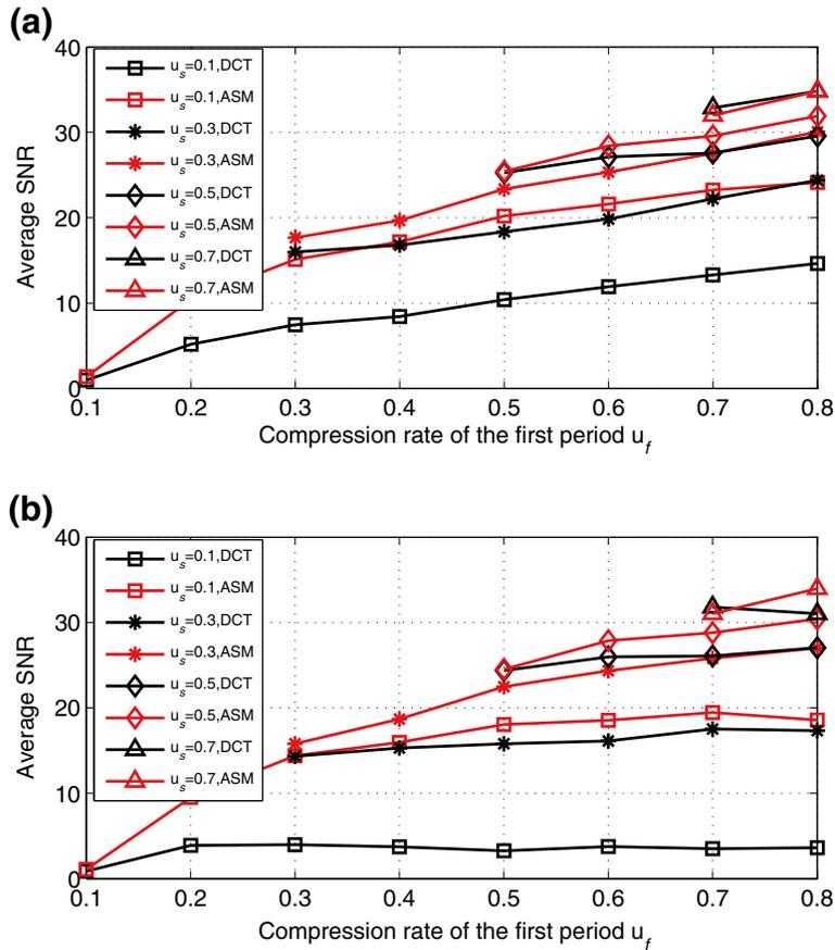
**Figure 6** Average SNR of voiced speech signals whose waveforms are similar to that in Figure 3a. (a) Average reconstruction SNR of pitch periods with different values of  $f u$  and  $s u$ . (b) Average reconstruction SNR of frames with different values of  $f u$  and  $s u$ .
