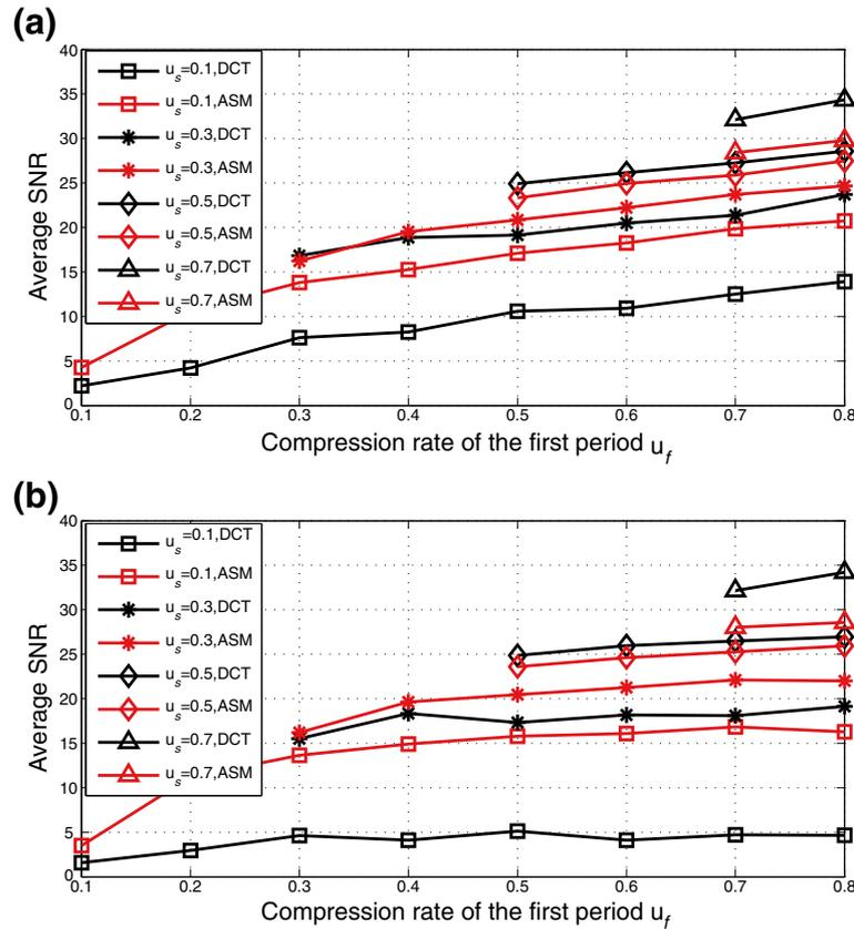
**Figure 5** Average SNR of voiced speech signals whose waveforms are similar to that in Figure 2a. (a) Average reconstruction SNR of pitch periods with different values of  $f u$  and  $s u$ . (b) Average reconstruction SNR of frames with different values of  $f u$  and  $s u$ .
