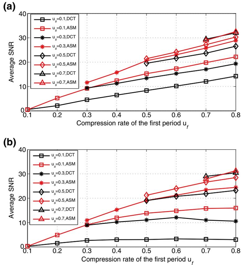
**Figure 4** Average SNR of voiced speech signals whose waveforms are similar to that in Figure 1 (a): (a) Average reconstruction SNR of pitch periods with different values of  $u_f$  and  $u_s$ . (b) Average reconstruction SNR of frames with different values of  $u_f$  and  $u_s$ . ASM in the figure stands for adaptive sparsifying matrix.
