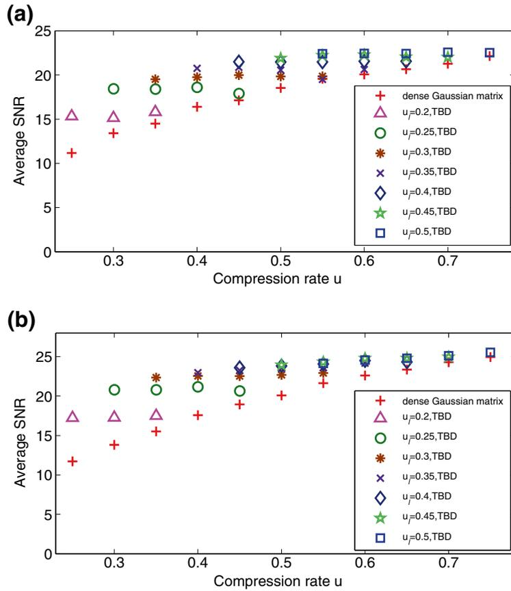
**Figure 15** Average SNR of adaptive quantization of entire speech signals with different quantization levels: (a)  $Q=32$ . (b)  $Q=64$ .
