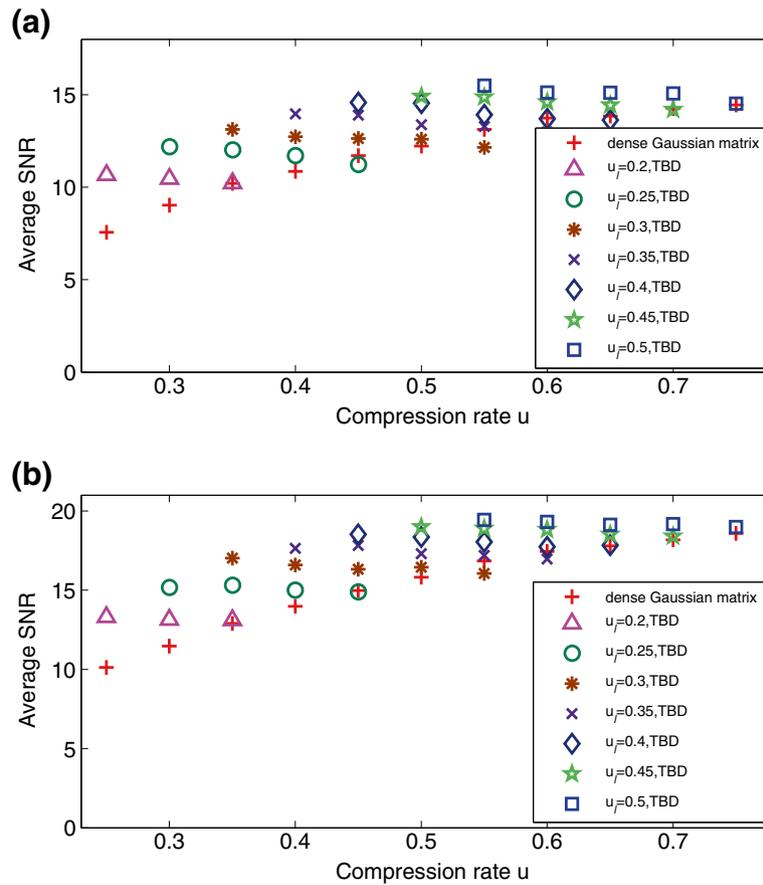
**Figure 14** Average SNR of adaptive quantization of entire speech signals with different quantization levels: (a)  $Q=8$ . (b)  $Q=16$ .
