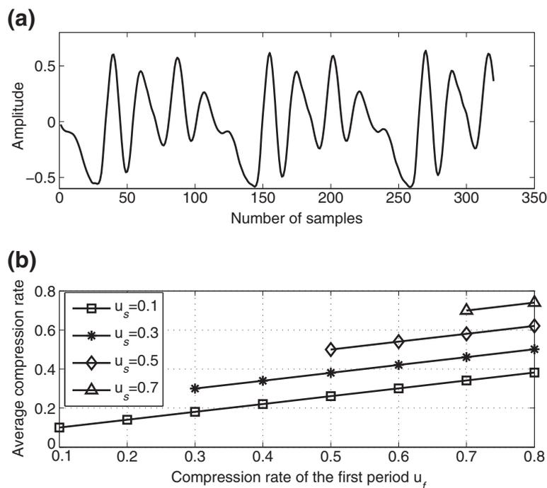
**Figure 1** Waveform of the first type of voiced speech signals and average compression rate: (a) Waveform of the first type of voiced speech signals. (b) Average compression rate with different values of  $u_f$  and  $u_s$ .
