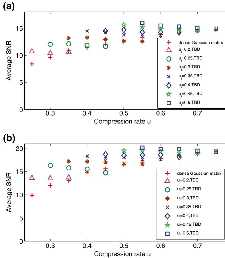
**Figure 12** Average SNR of adaptive quantization of voiced speech signals with different quantization levels: (a)  $Q=8$ . (b)  $Q=16$ .
