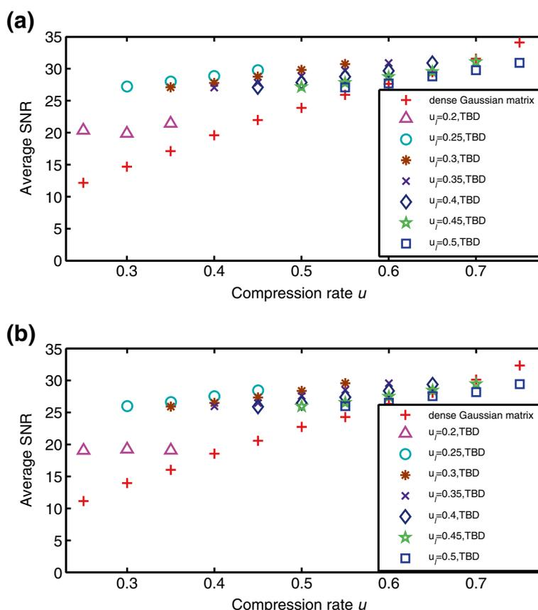
**Figure 10** Comparison of average SNR between the TBD matrix and the dense Gaussian matrix: (a) Average reconstruction SNR of voiced speech signals when the sparsifying matrix is the DCT basis. (b) Average reconstruction SNR of the entire speech signals when the sparsifying matrix is the DCT basis.
