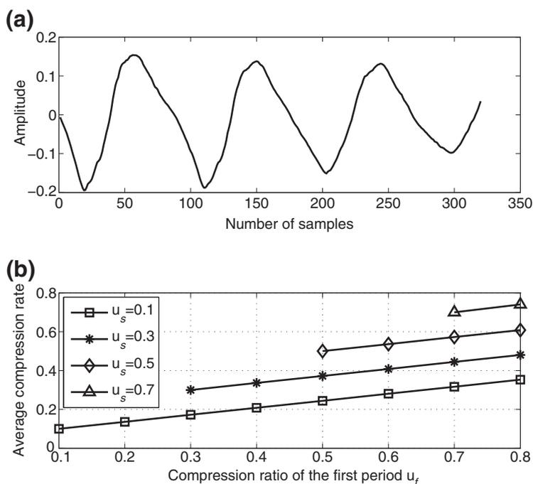
**Figure 2** Waveform of the second type of voiced speech signals and average compression rate: (a) Waveform of the second type of voiced speech signals. (b) Average compression rate with different values of  $u_f$  and  $u_s$ .
