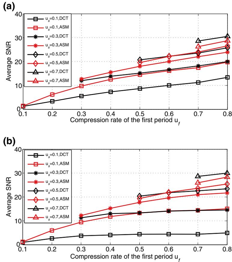
**Figure 8** Average SNR of the entire speech signals: (a) Average reconstruction SNR of pitch periods with different values of  $u_f$  and  $u_s$ . (b) Average reconstruction SNR of frames with different values of  $u_f$  and  $u_s$ . ASM in the figure stands for adaptive sparsifying matrix.
