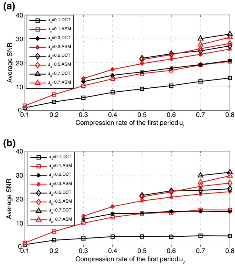
**Figure 7** Average SNR of all the voiced speech signals in the testing speech signals: (a) Average reconstruction SNR of pitch periods with different values of  $u_f$  and  $u_s$ . (b) Average reconstruction SNR of frames with different values of  $u_f$  and  $u_s$ . ASM in the figure stands for adaptive sparsifying matrix.
