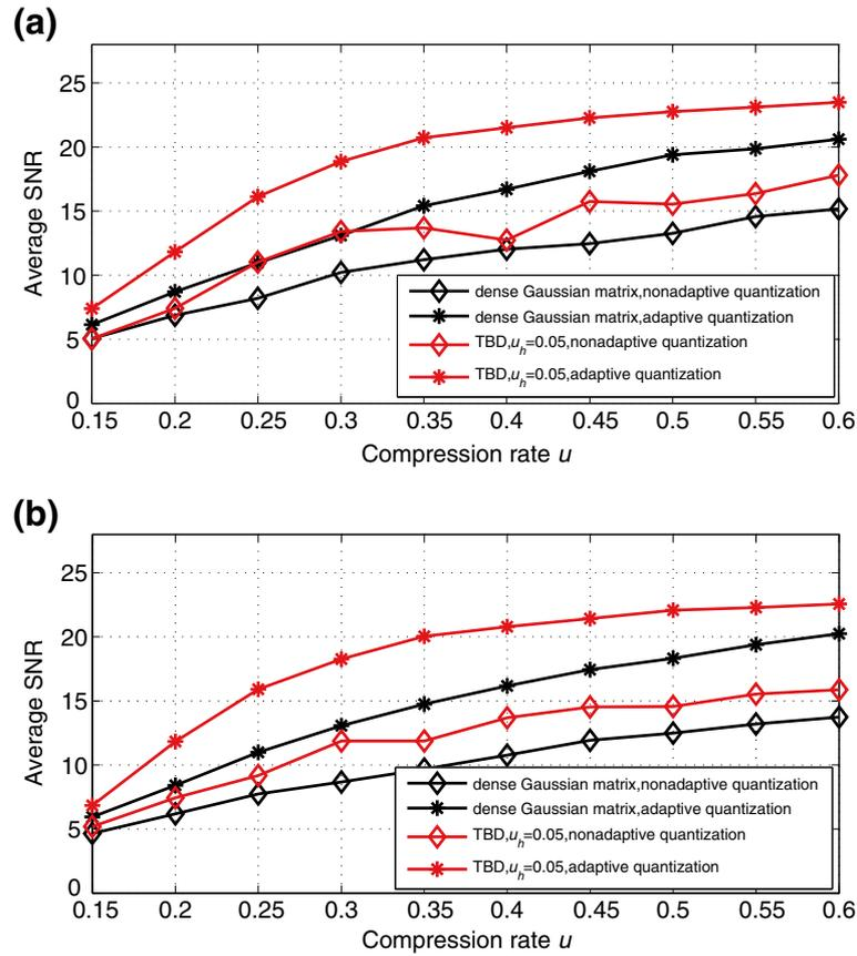
**Figure 11** Average reconstruction SNR of adaptive quantization and nonadaptive quantization: (a) Average reconstruction SNR of voiced speech signals with respect to the TBD matrix and dense Gaussian matrix in the case of adaptive quantization and nonadaptive quantization. (b) Average reconstruction SNR of the entire testing speech signals with respect to the TBD matrix and dense Gaussian matrix in the case of adaptive quantization and nonadaptive quantization.
