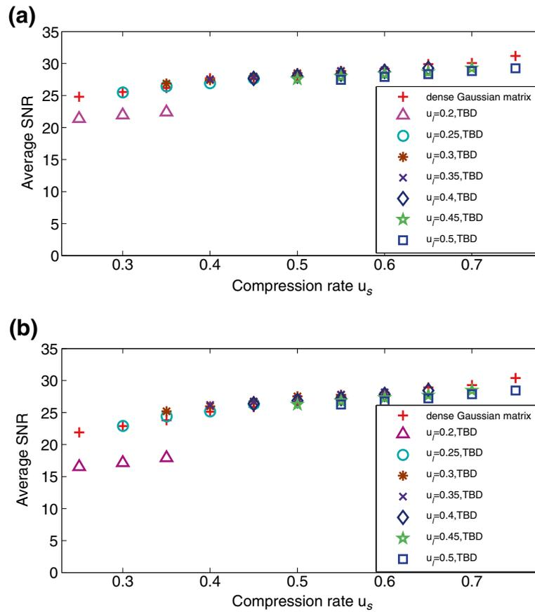
**Figure 9** Comparison of average SNR between the TBD matrix and the dense Gaussian matrix: (a) Average reconstruction SNR of pitch periods of voiced speech signals with respect to the adaptive sparsifying matrix. (b) Average reconstruction SNR of frames of voiced speech signals with respect to the adaptive sparsifying matrix.
