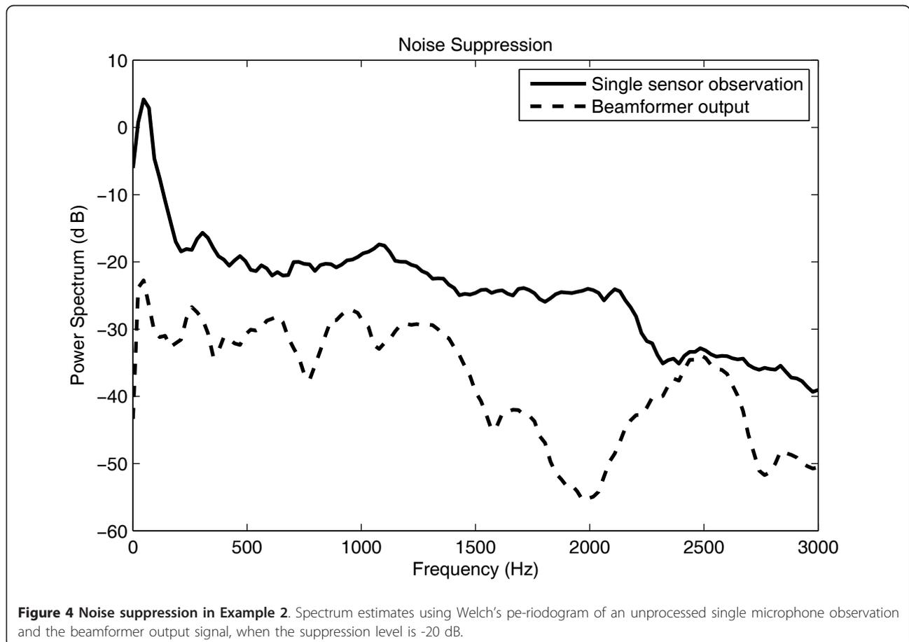
**Figure 4 Noise suppression in Example 2.** Spectrum estimates using Welch's pe-riodogram of an unprocessed single microphone observation and the beamformer output signal, when the suppression level is -20 dB.
