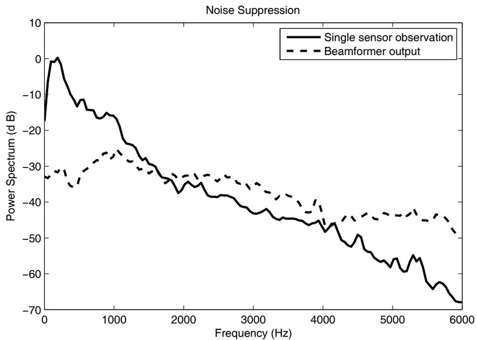
**Figure 3** Interference suppression in Example 1. Spectrum estimates using Welch's periodogram of an unprocessed single microphone observation and the beamformer output signal, when the distortion level is -20 dB.
