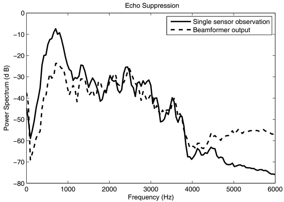
**Figure 2** Noise suppression in Example 1. Spectrum estimates using Welch's pe-riodogram of an unprocessed single microphone observation and the beamformer output signal, when the distortion level is -20 dB.
