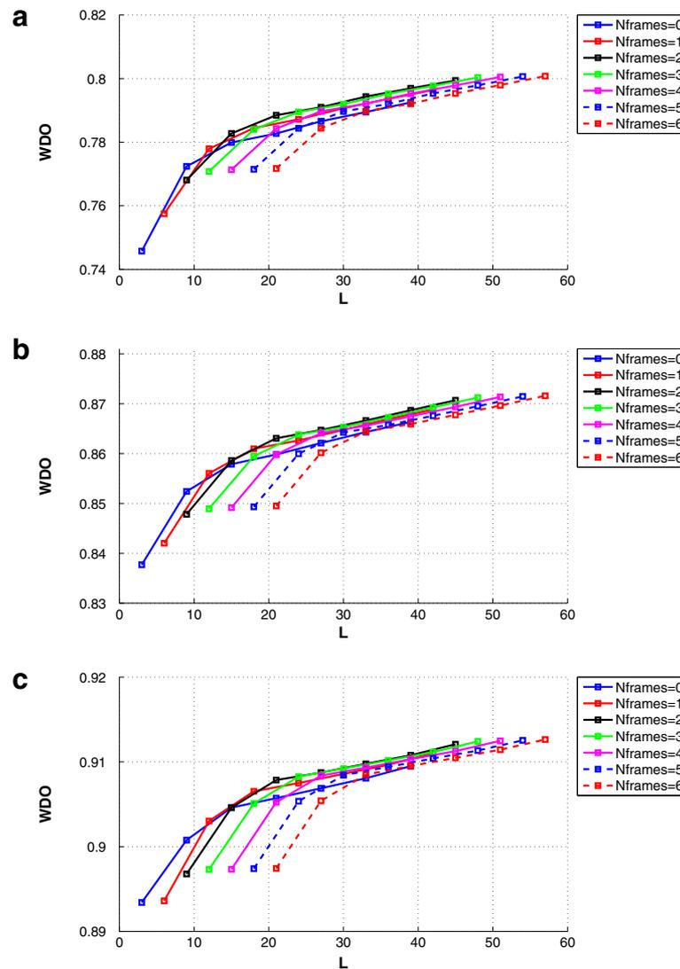
**Figure 4 Time-frequency footprint selection.** (a) SNR = 0 dB, (b) SNR = 3 dB and (c) SNR = 5 dB. Description: average WDO value obtained by the non-quantified classifier with the selected combination of features varying the number of neighbor frequencies (*Nfreqs*) and previous time frames (*Nframes*) of the time-frequency footprint. The different values of *Nframes* are represented with lines of different colors and the different values of *Nfreqs* with squares over the lines.
