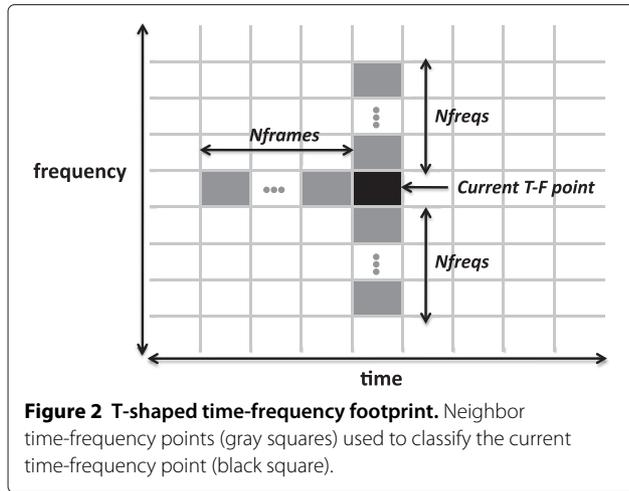
The experiments carried out in this section have two objectives: first, the selection of the best set of features among the six proposed (Table 1) and second, the selection of the optimum time-frequency footprint, finding the best values for  $Nfreqs$  and  $Nframes$ . The two problems are solved separately in two different experiments described below.
