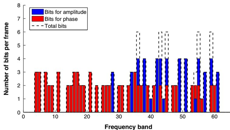
**Figure 6 Bit distribution among frequency bands.** Distribution of the number of bits per frame among the frequency bands, in the case of a transmission rate of 64 kbps and SNR of 0 dB. The blue bars represent the number of bits assigned to the amplitude values ( $B_{AK}$ ), the red bars represent the number of bits assigned to the phase values ( $B_{PK}$ ), and the dashed black line the total number of bits assigned to each frequency band ( $B_{AK} + B_{PK}$ ).
