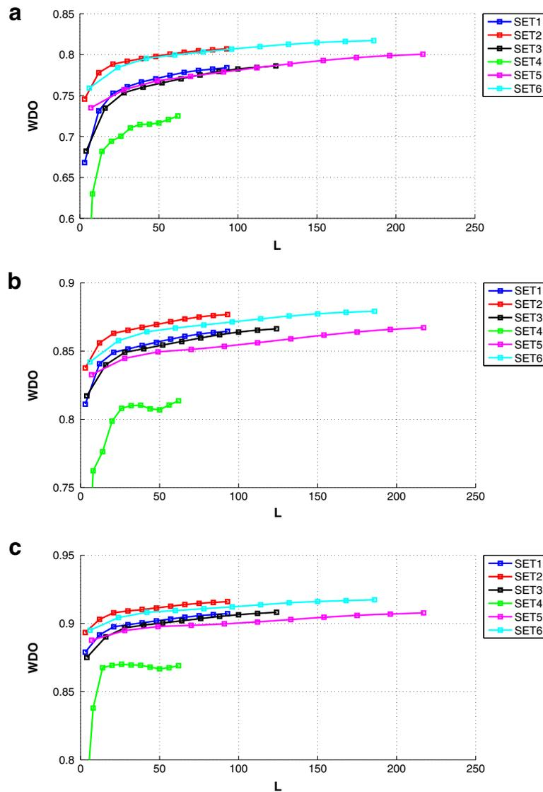
**Figure 3 Feature selection.** (a) SNR = 0 dB, (b) SNR = 3 dB, and (c) SNR = 5 dB. Average WDO value obtained by the non-quantified classifier using different combinations of features and different sizes of the time-frequency footprint, with  $N_{freqs} = N_{frames}$ . The different set of features are represented with lines of different colors, and the different values of  $N_{freqs}$  (and  $N_{frames}$ ) are represented with squares over the lines.
