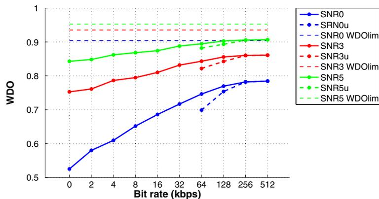
**Figure 5 WDO vs. bit rate.** WDO values averaged over the test set as a function of the transmission bit rate (kbps) obtained by the proposed transmission schema in the case of an optimized distribution of bits (solid line) and a uniform distribution of bits (dashed line). The different colors represent different SNR values. The limiting WDO value ( $WDO_{lim}$ ) is represented by a straight line for each SNR.
