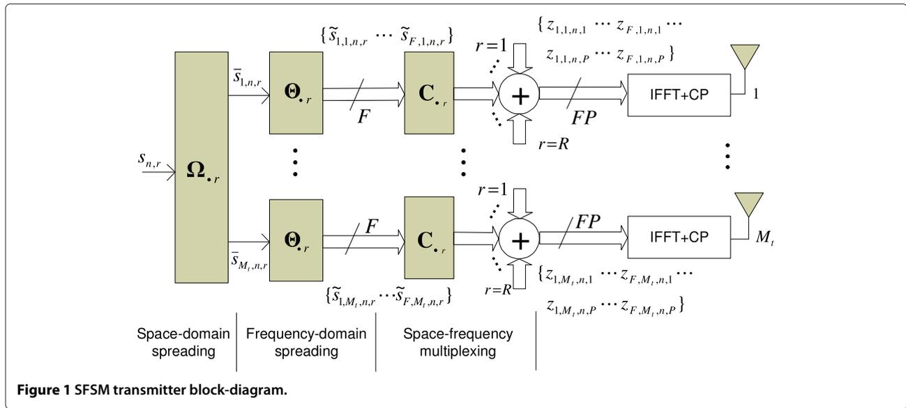
**Figure 1** SFSM transmitter block-diagram.
