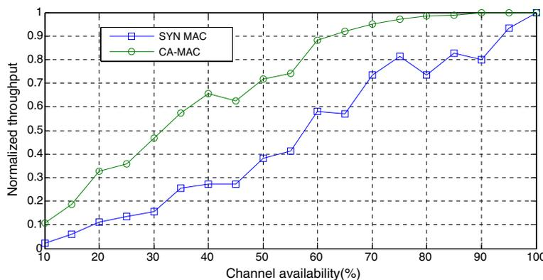
Figure 13 Network throughput at different channel availability.
