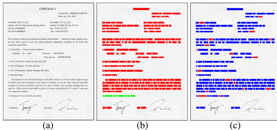
Figure 10 Tampered document (a contract) and its detection results. (a) The document tampered by add-printing or splice-copying, (b) the detection result for add-printing, and (c) the detection result for splice copying.
