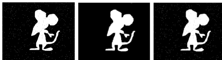
Figure 16 Example of binary image filtered respectively by the AGK and the static filter.
