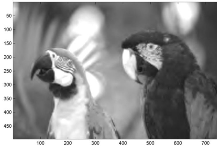
Figure 9 Simulated LR reference frame. This is after individual-frame JPEG2000 compression (CR = 8) and then L = 4 bicubic interpolation.
