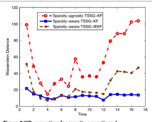
**Figure 8** WD versus time for sparsity-agnostic and sparsity-aware TSSG-KF and TSSG-IEKF trackers.
