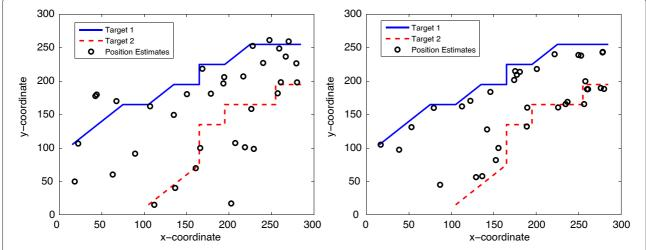
**Figure 7 True tracks and position estimates for two targets.** Sparsity-agnostic TSSG-KF tracker (left) and sparsity-aware TSSG-KF tracker (right). Circles indicate the estimated target positions.
