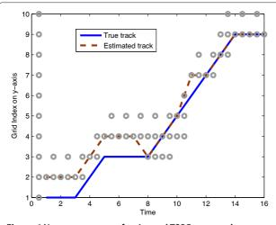
**Figure 6** Nonzero support of estimated TSSG, true, and estimated tracks (*y*-direction only).
